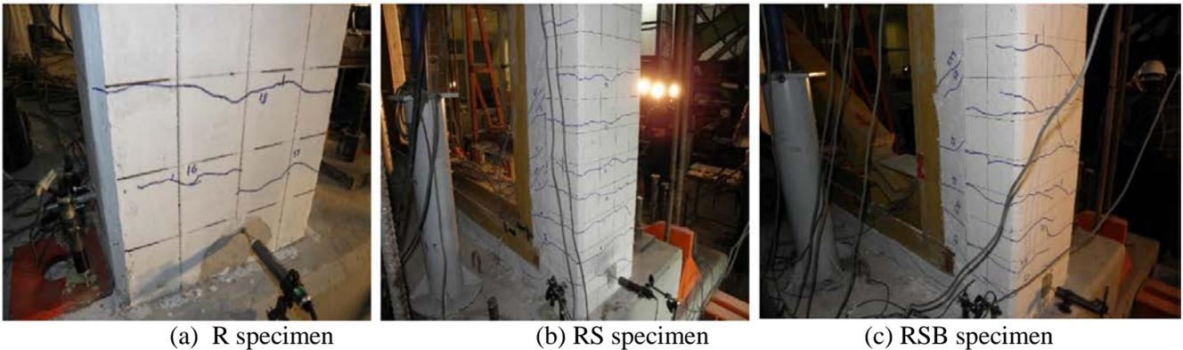
Fig. 8. Damage at North column bottom end at retrofit target story drift angle (1/150)
