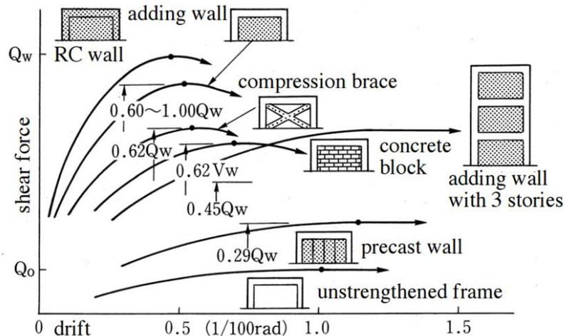
Figure 1. Retrofitting methods for seismically deficient RC frames [1]
