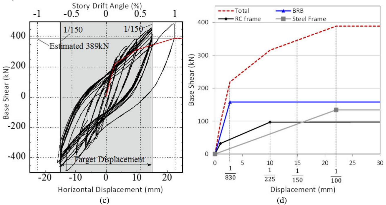
Fig. 7. Load versus drift responses of (a) R model: Bare RC frame (b)RS model: RC frame with steel frame (c) RSB model: RC frame with steel frame and BRB (d) Estimated push-over behavior of RSB model.
