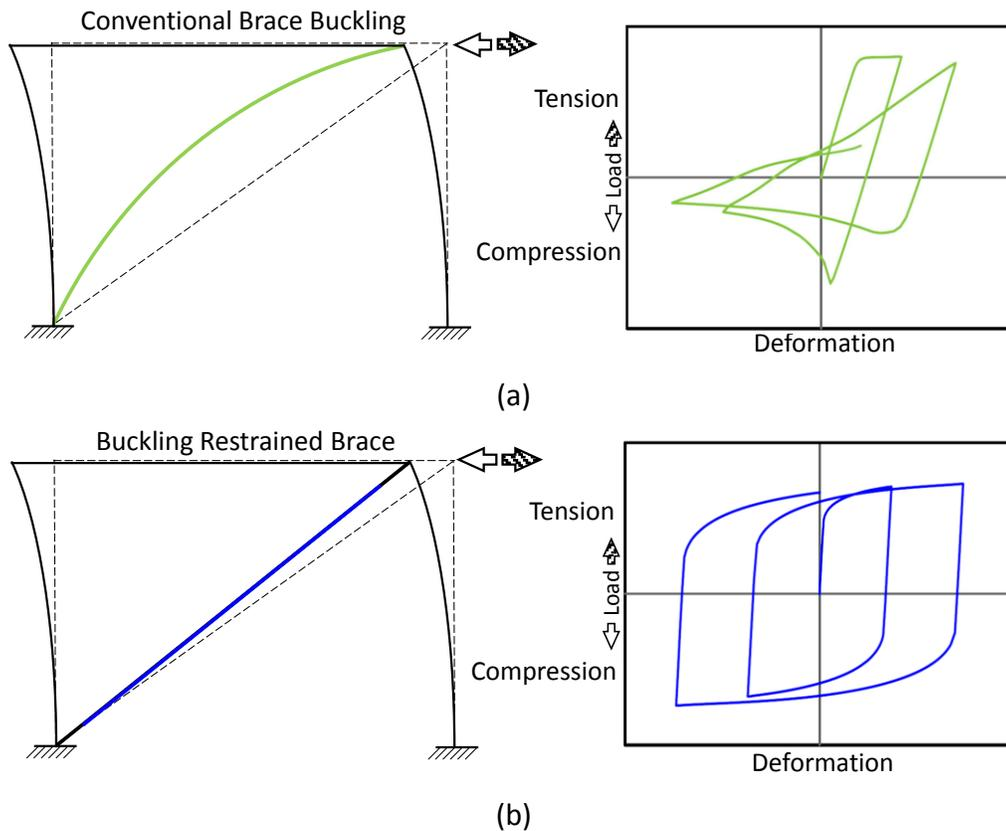
Fig. 2. Seismic behavior of frame with conventional steel brace (a) and BRB (b)
