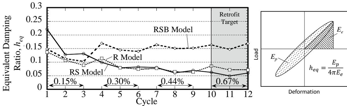
Fig. 11. Comparison of equivalent damping ratio (until retrofit target story drift angle of 1/150)
