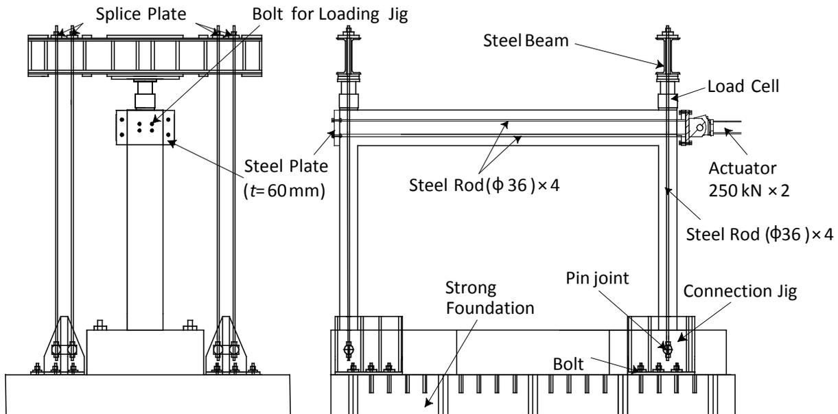
Fig. 6. Horizontal Cyclic and Axial Load System
