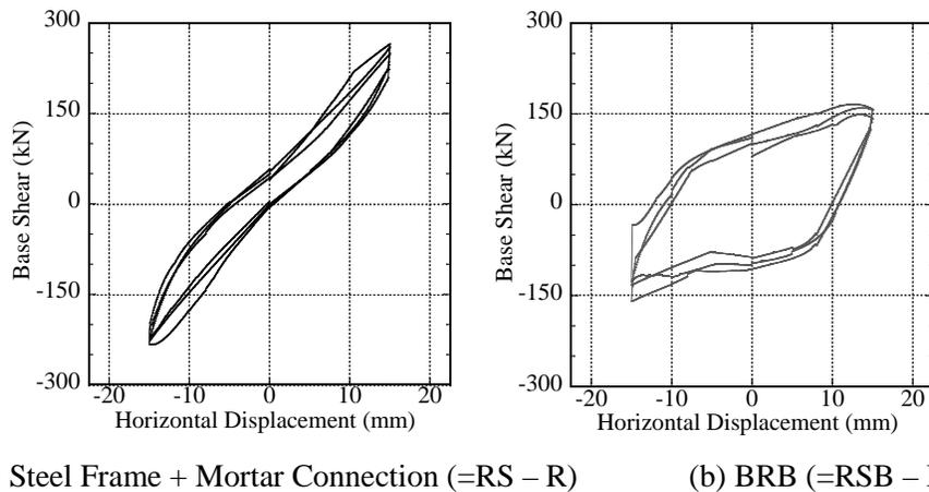
Fig. 9. Load-displacement relationships of steel frame and BRB at target story drift cycles (1/150)
