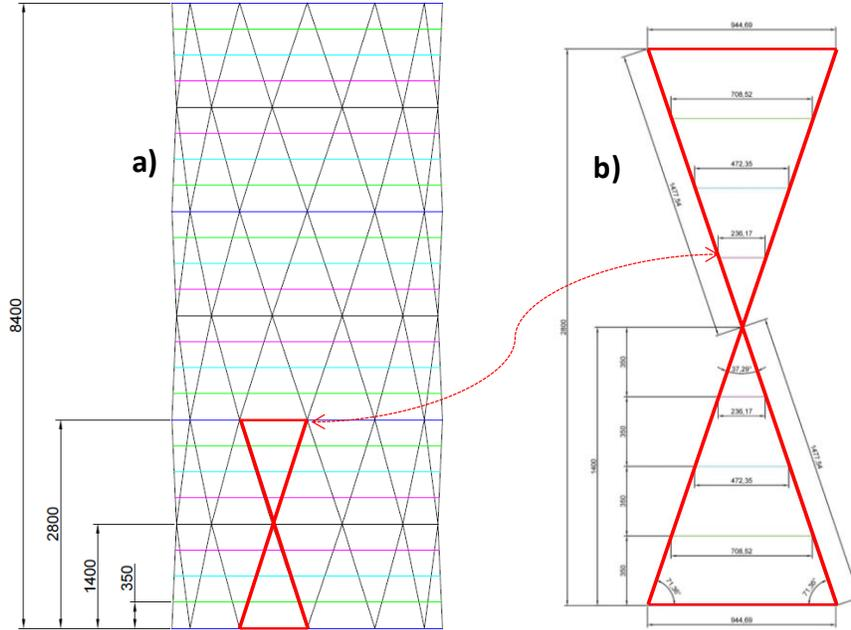
Fig.4 - Elevation views of 24-story building: a) Diagrid; b) Triangular module
