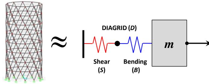
Fig.1 - Equivalent single-degree-of-freedom system
