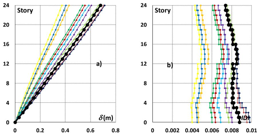
Fig.8 - Distributions of lateral deformation along height, nonlinear dynamic analyses: a) Story displacement; b) Interstory drift index
