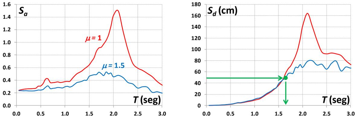
Fig.5 - Design spectra,  $\xi = 0.05$ : a) Strength; b) Displacement
