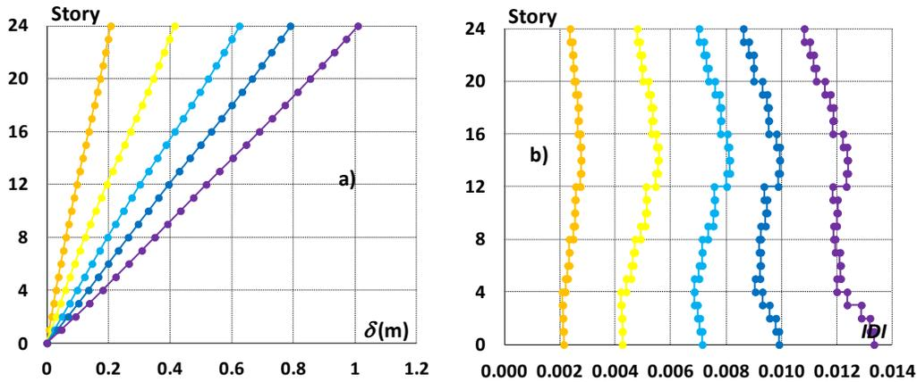
Fig.7 - Distributions of lateral deformation along height, nonlinear static analysis: a) Story displacement; b) Interstory drift index
