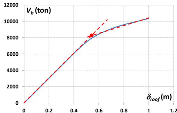
Fig.6 - Capacity curve of 24-story building
