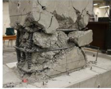
Beam 1 – Failed by fracture of longitudinal bars Beam 2 – Failed by buckling of longitudinal bars Fig. 7: Failure mechanism of Beams 1 & 2.
