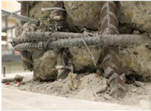
Beam 1 – Failed by fracture of longitudinal bars Beam 2 – Failed by buckling of longitudinal bars Fig. 7: Failure mechanism of Beams 1 & 2.
