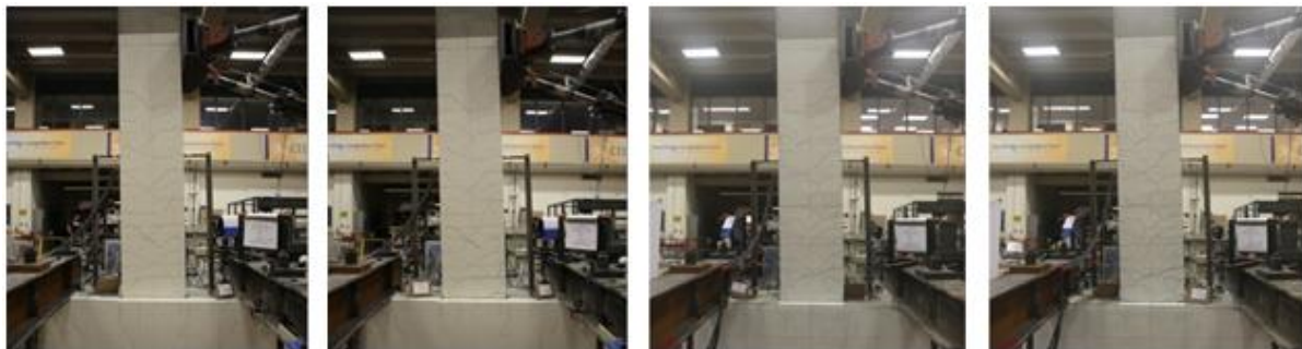
Beam 1 – at 1.96\Delta y Beam 1 – at 2.75\Delta y Beam 2 – at 1.96\Delta y Beam 2 – at 2.75\Delta y
