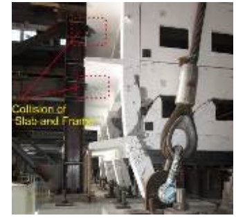
(c) Collision with steel frame
