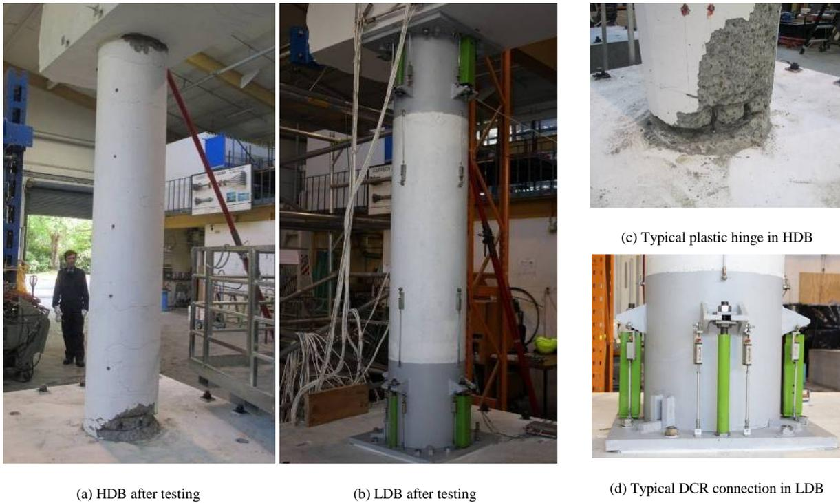
Fig. 13– Damage to HDB and LDB following testing
