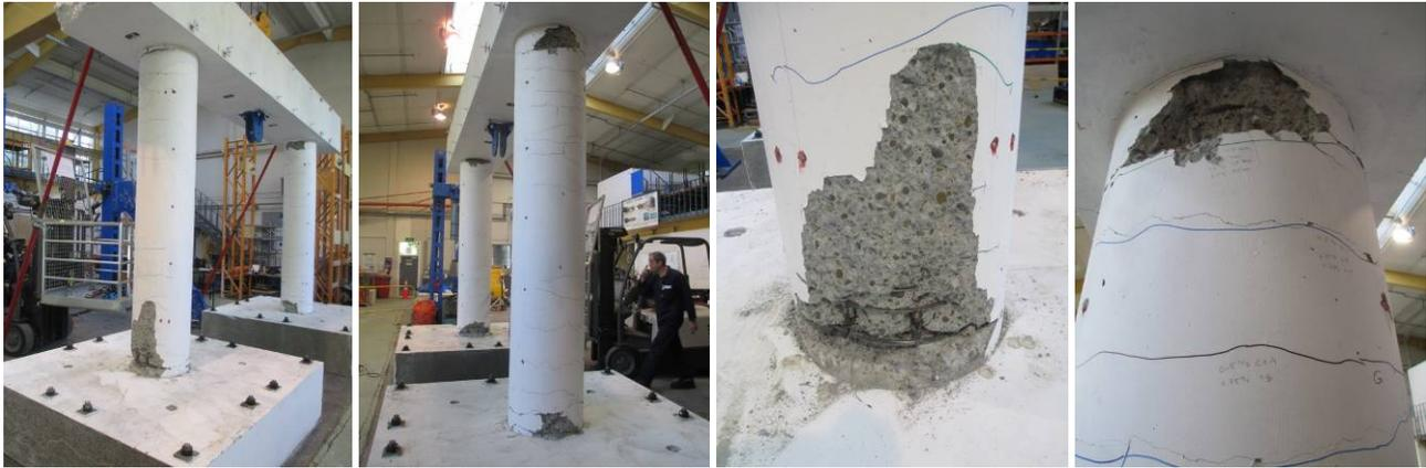
(a) Plastic hinges in the columns of HDB following uniaxial cyclic testing      (b) Typical bottom MSC      (c) Typical top GDC
