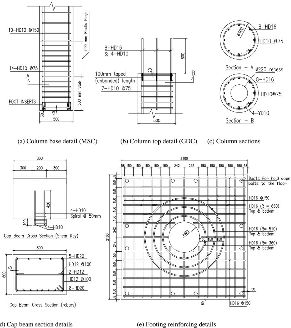
Fig. 6– Reinforcing details of precast elements for HDB
