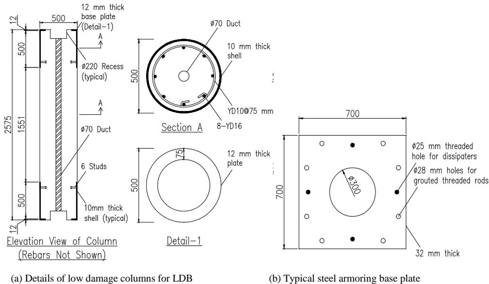
Fig. 9– Reinforcing details of precast columns for LDB
