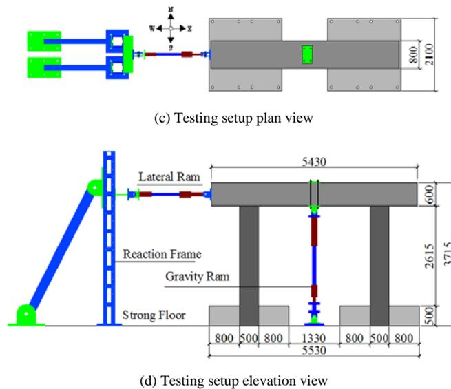
Fig. 5– Loading protocol and testing setup
