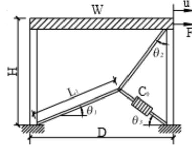
Fig. 4 – Installation of Lower Toggle Brace system [1]
