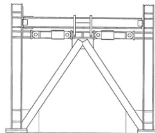
Fig. 2 – Installation of Chevron Damper
