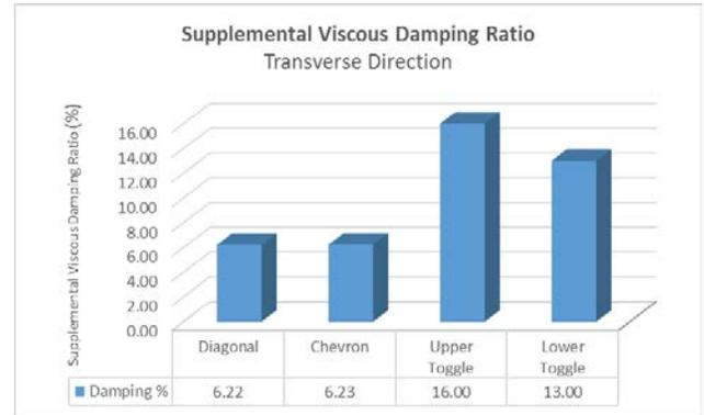
Fig. 16 – Damping Ratio - Transverse Direction
