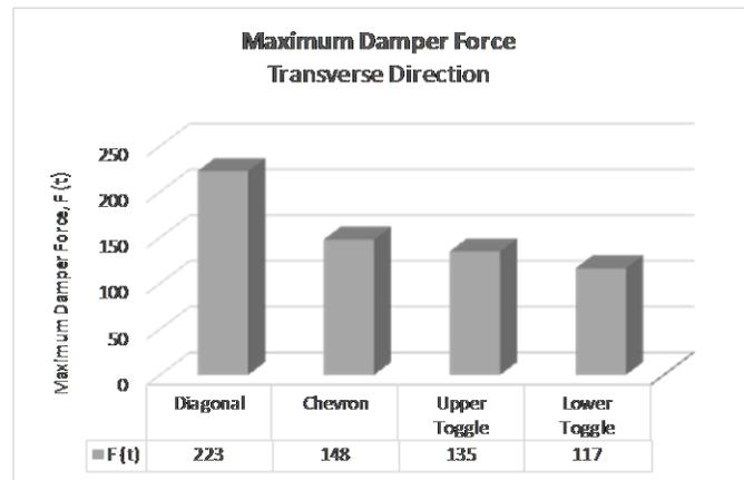
Fig. 18– Maximum Damper Force of Transverse Direction
