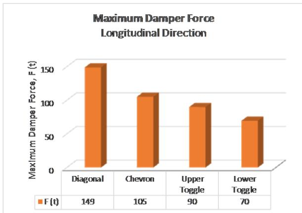
Fig. 17 – Maximum Damper Force of Longitudinal Direction
