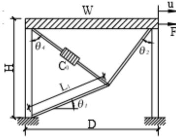
Fig. 3 – Installation of Upper Toggle Brace system [1]
