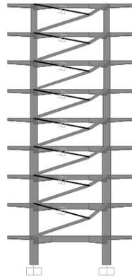
Fig. 9 – Upper Toggle Brace – Longitudinal Direction
