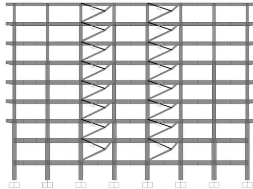
Fig. 10 – Upper Toggle Brace Transverse Direction
