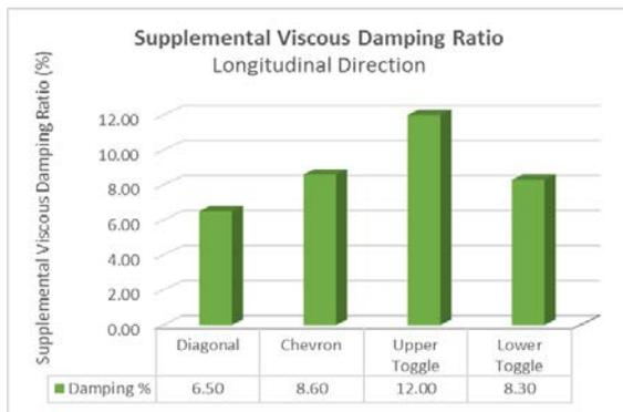
Fig. 15 – Damping Ratio – Longitudinal Direction
