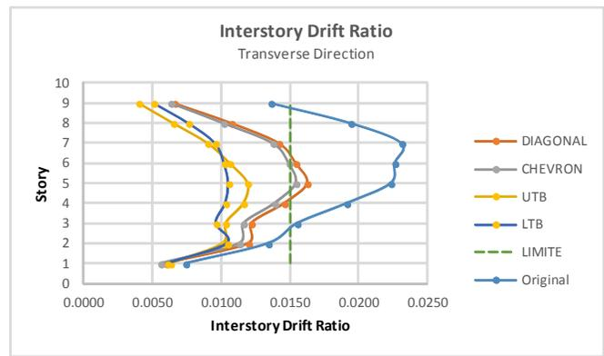
Fig. 12 – Interstory Drift Ratio - Transverse Direction
