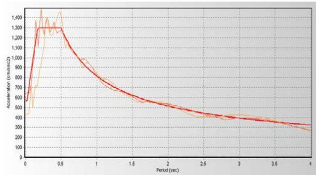
Fig. 8 – Earthquake response spectra generated by ground motions compatible with design spectrum
