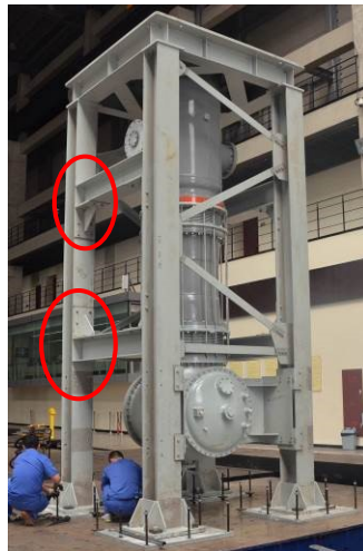
(a) The construction of Frame-O
