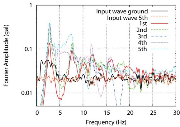
(a) Fourier amplitude spectra for input and response motions
