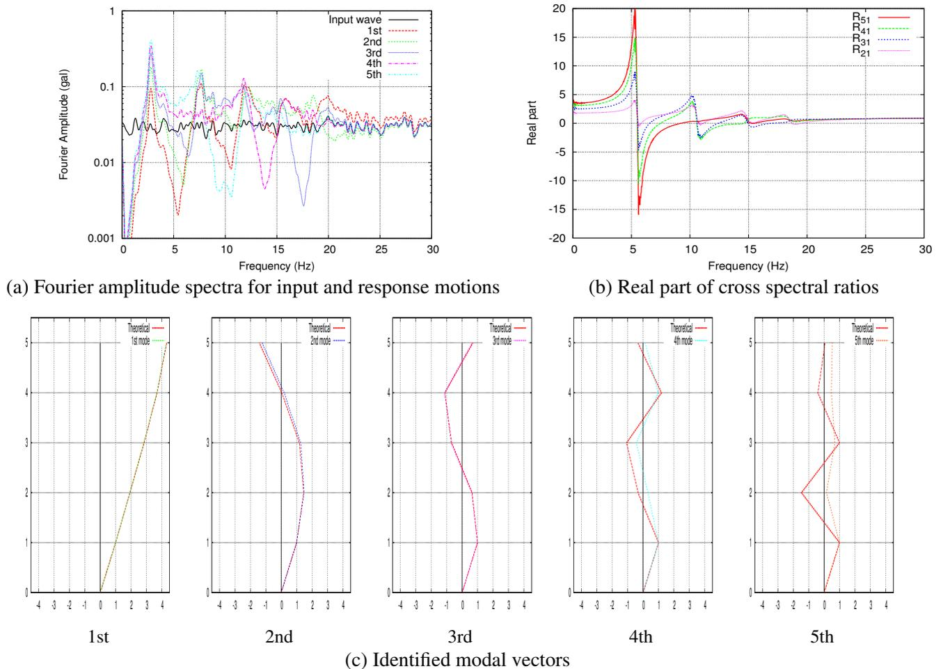
Fig. 2 – Modal parameters identified through the proposed method (Case 1).
