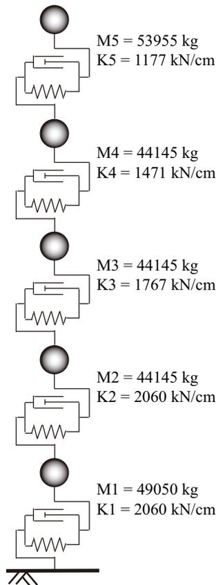
**Fig. 1** A model of 5DOF system for numerical simulation.
