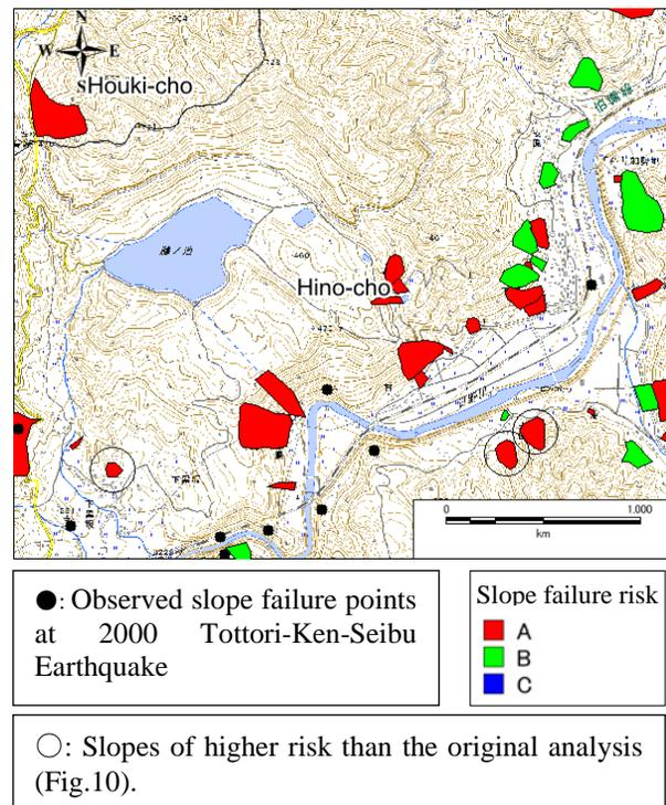
Fig. 14 - Risk assesment map of earthquake induced slope failure regarding 3D topographic effect.
