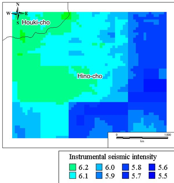
Fig. 13 - Instrumental seismic intensity distribution corrected by 3D topographic effect formula (3) ( $I_{jma50}'$ ).
