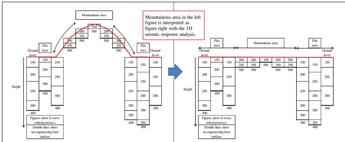
Fig. 15 - The schematic diagram of approximation when mountainous area is expressed approximately in 1D ground analysis model.
