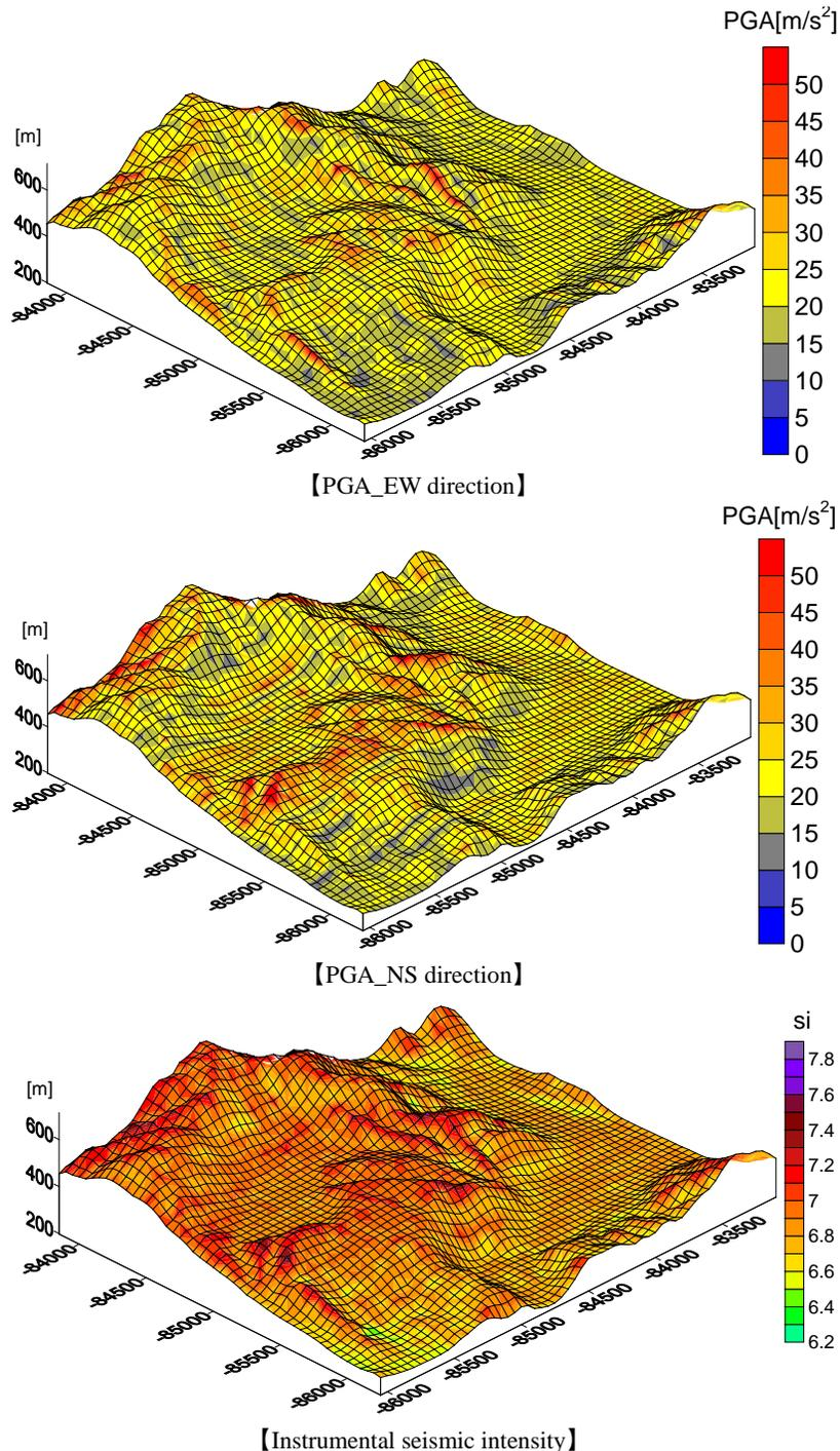
Fig. 9 - 3D view of surface peak ground acceleration (PGA) and instrumental seismic intensity (si) in 50m grid cells by BESSRA 3D-FEM seismic response analysis results.
