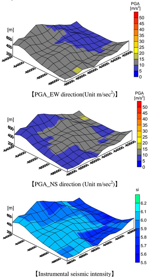
Fig. 6 - 3D view of surface peak ground accelerations (PGA) and instrumental seismic intensity (si) in 250m grid cells by seismic micro-zoning survey.
