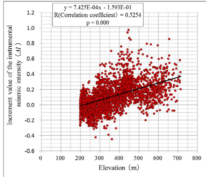
Fig. 11 - Correlation between the increment of the instrumental seismic intensity and the elevation of the 50m grid cells.
