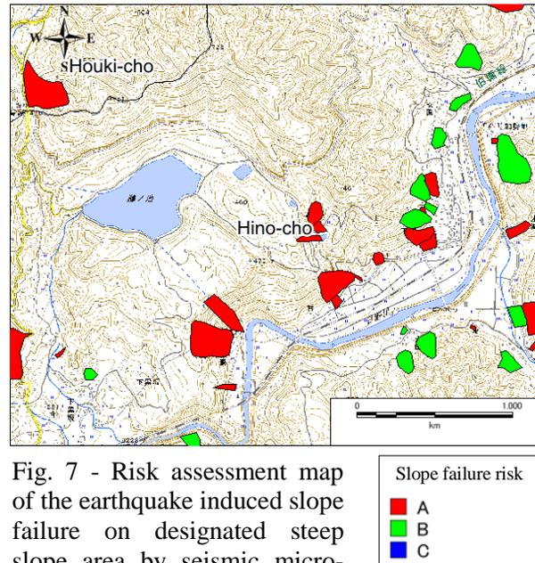
Fig. 7 - Risk assessment map of the earthquake induced slope failure on designated steep slope area by seismic micro-zoning technique<sup>[11]</sup>.
