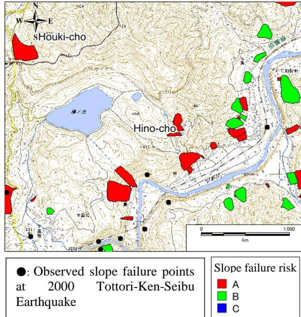
Fig. 10 - Distribution of the observed slope failure points at the 2000 Tottori-Ken-Seibu Earthquake with the assessed slope failure ranks on seismic micro-zoning.
