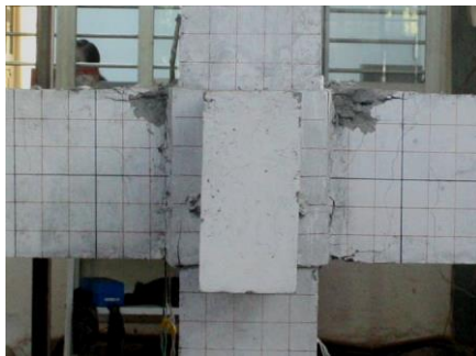
(c) Retrofitted specimen J3
