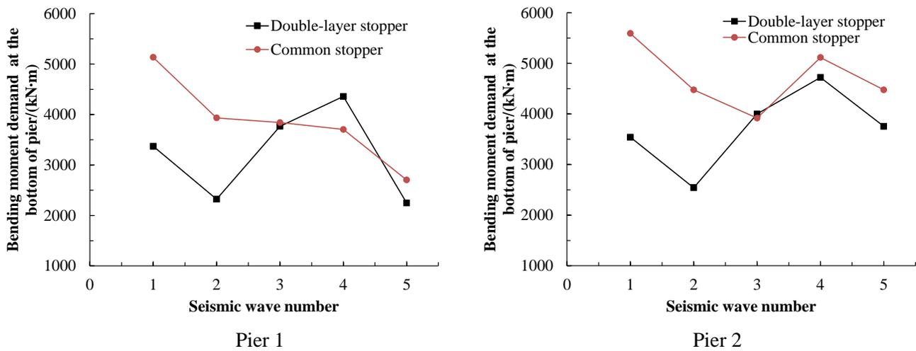
Fig. 7 –Maximum bending moment demands at the bottom of piers
