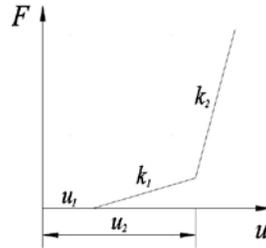
Fig. 2 –Contact element restoring model
