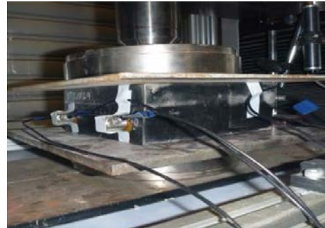
Fig. 3 – Locations of AE sensors (Left) and View of the experiment (Right)
