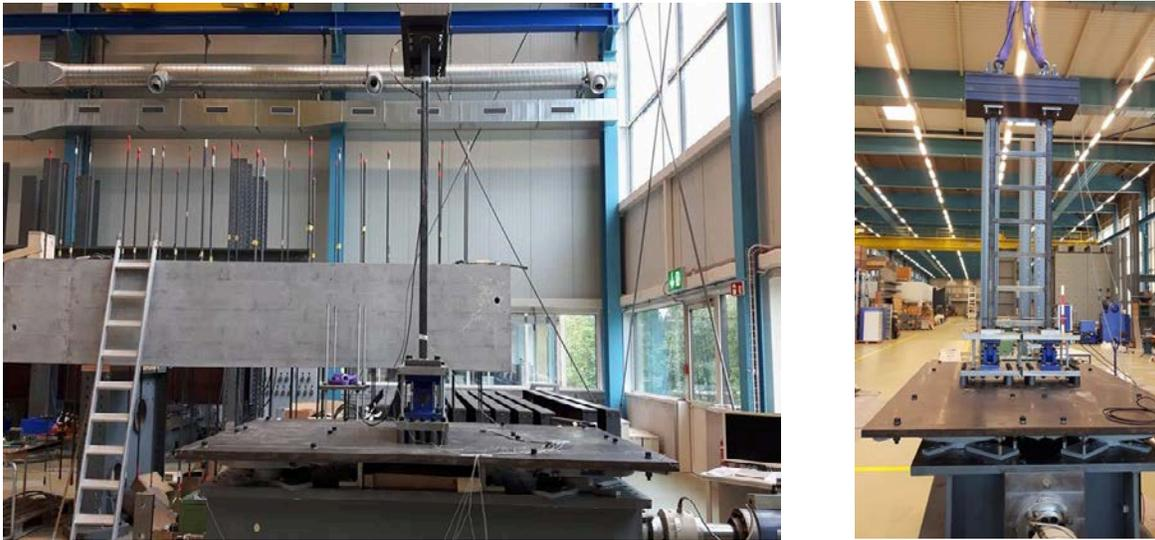
Fig. 4: Constructed isolated structure in the ETH laboratory
