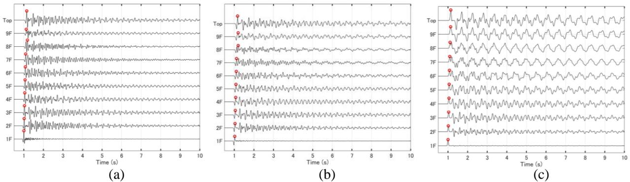
Fig. 3 – Response of the MDOF model to the input Ricker Wavelet; (a) is acceleration, (b) is the velocity, and (c) is the displacement response waveforms
