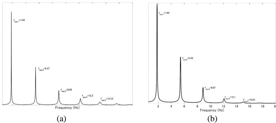
Fig. 5 – (a) transfer function between the displacement response of the top and the base; (b) spectrum of the displacement response of the top
