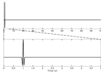
Fig. 2 – incident wave to the MDOF model
