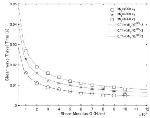
Fig. 10 – change of shear-wave travel time with the increasing shear rigidity
