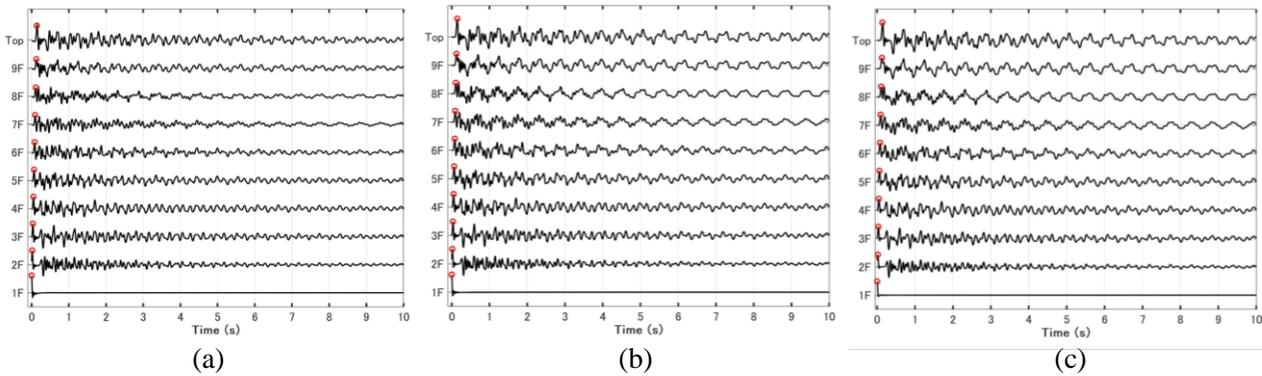
Fig. 4 – Impulse response of the MDOF model; (a) is acceleration, (b) is the velocity, and (c) is the displacement response waveforms
