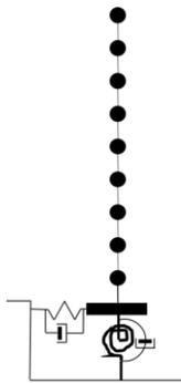
Fig. 1 – MDOF model with rocking and horizontal
