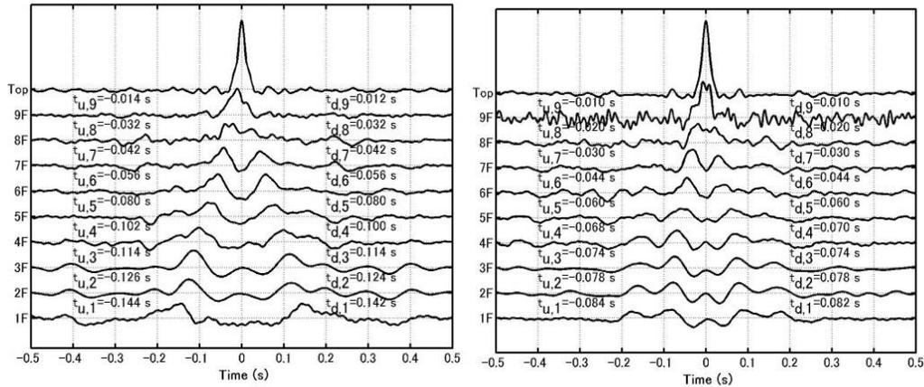
Fig. 11 - Deconvolved waves of Building QM in the longitudinal direction (left figure) and the transverse direction (right figure)
