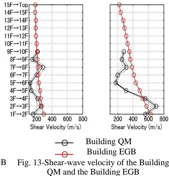
Fig. 13- Shear-wave velocity of the Building QM and the Building EGB
