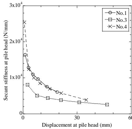
Fig. 6 – Lateral resistance of severely damaged piles (No.3, 4)
