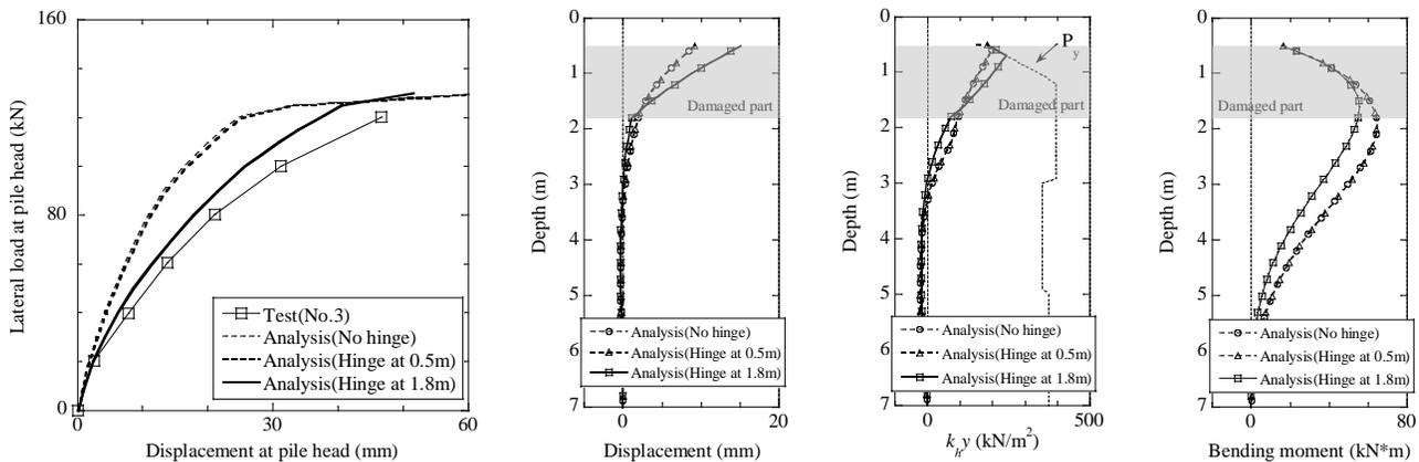
(a) Pile head load-displacement curves (b) Displacement (c) Subgrade reaction (d) Bending moment
