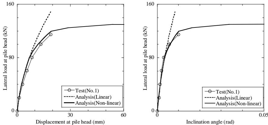
Fig. 12 – Lateral resistance of fine piles calculated from analyses (No.1)
