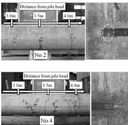
Photo. 1 – Pile damage
