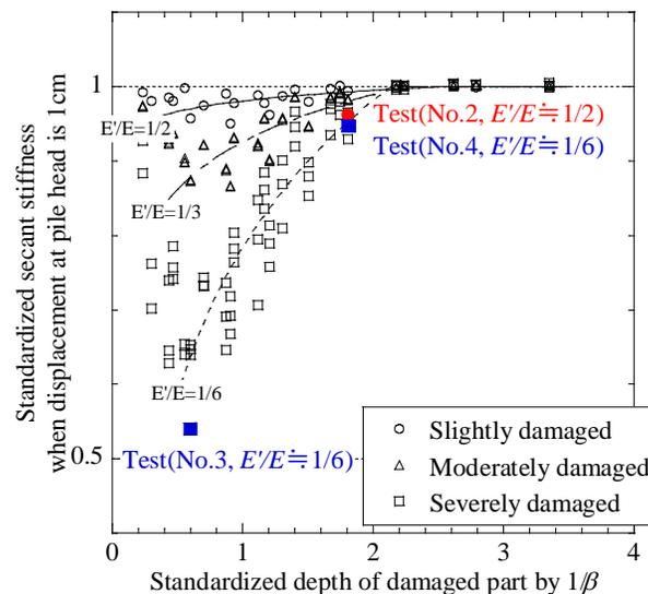
Fig. 16 – Evaluation of lateral resistance of damaged piles according to depth and extent of damage
