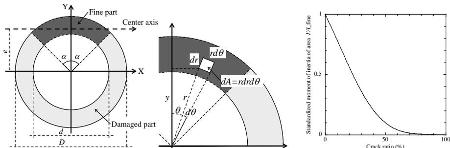
Fig. 10 – Method for calculating moment of inertia of area  $I'$  Fig. 11 – Moment of inertia of area  $I'$
