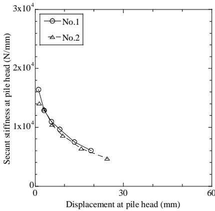
Fig. 5 – Lateral resistance of slightly damaged pile (No.2)
