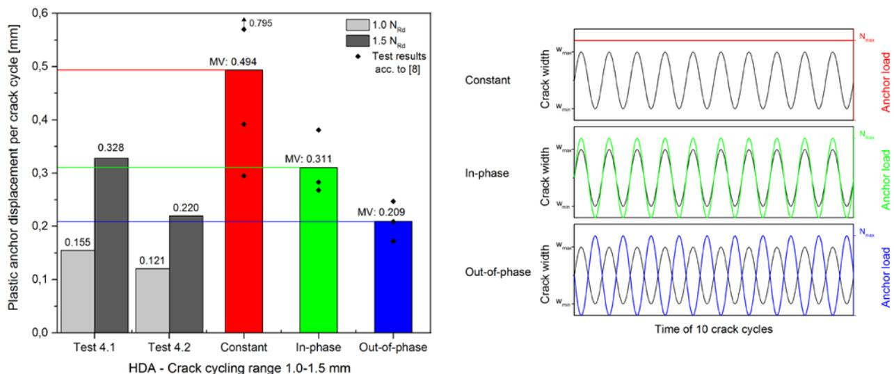
Fig. 13 – Comparison of plastic displacements for HDA anchors during tests with cycling crack width in the range of 1.0-1.5 mm (left) and loading protocol for tests on HDA anchors (right) with reference to [8]
