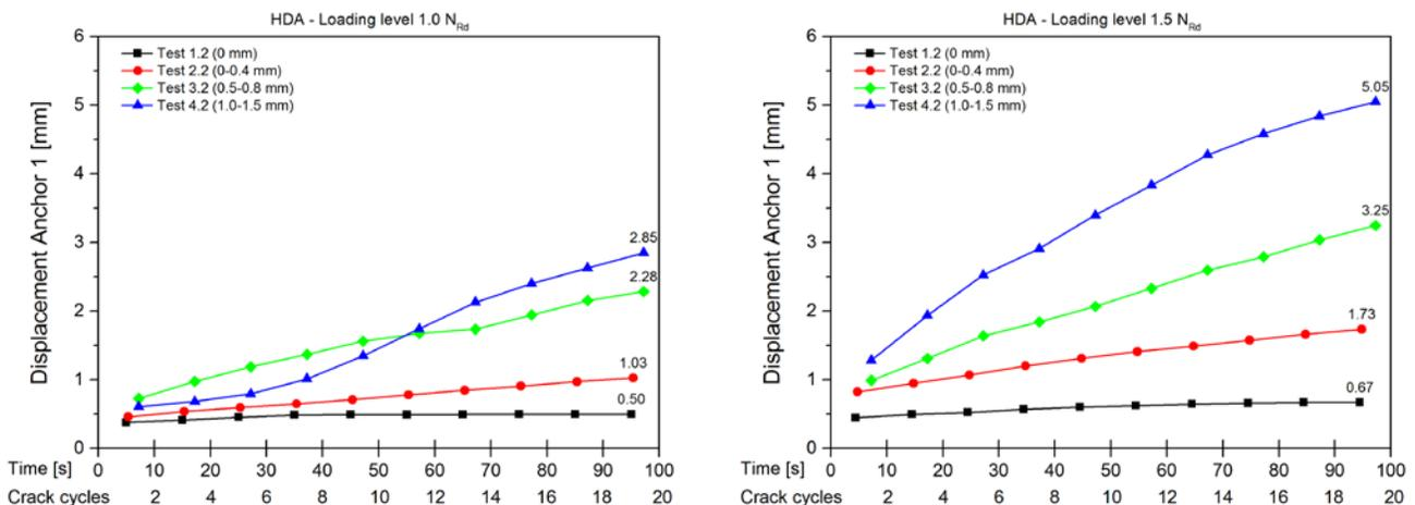
Fig. 12 – Comparison of anchor displacements at maximum anchor load: 1.0  $N_{Rd}$  (left) versus 1.5  $N_{Rd}$  (right)
