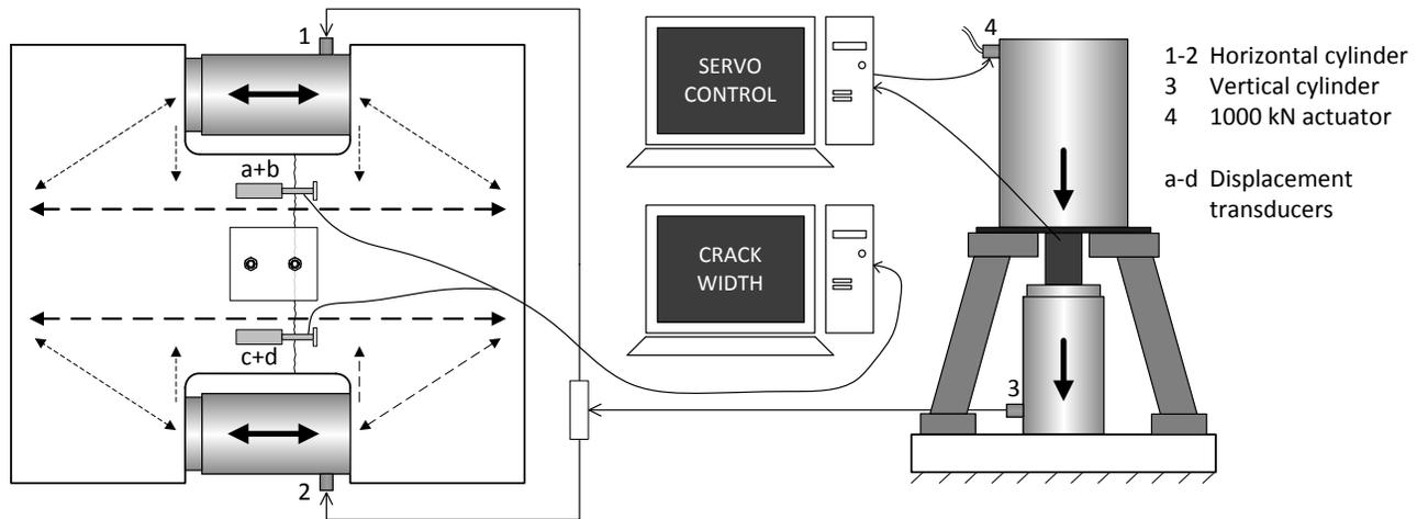
Fig. 6 – Test configuration for crack cycling
