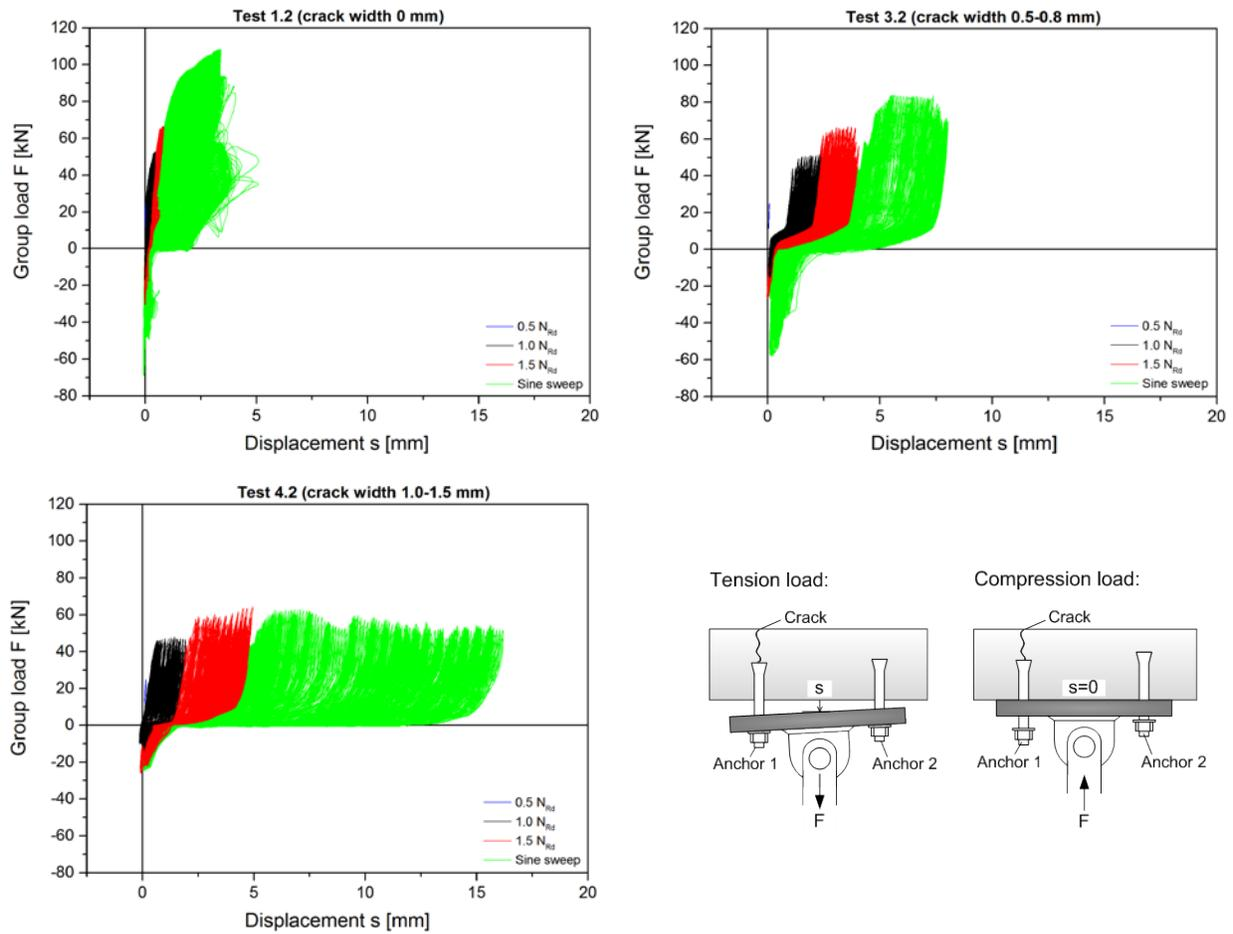
Fig. 7 – Load-displacement behavior of anchorage
