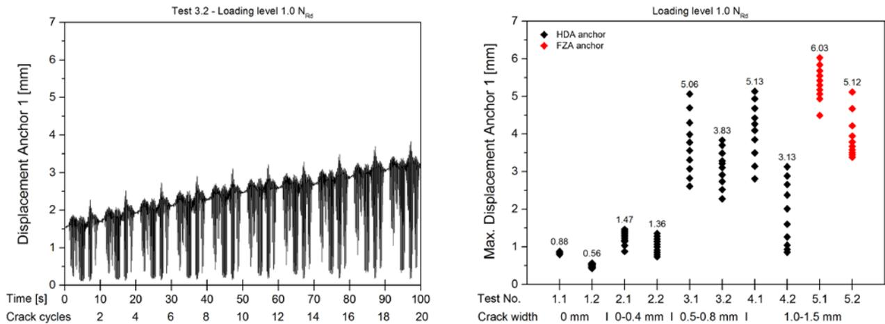
Fig. 11 – Displacements of Anchor 1 at loading level 1.0  $N_{Rd}$
