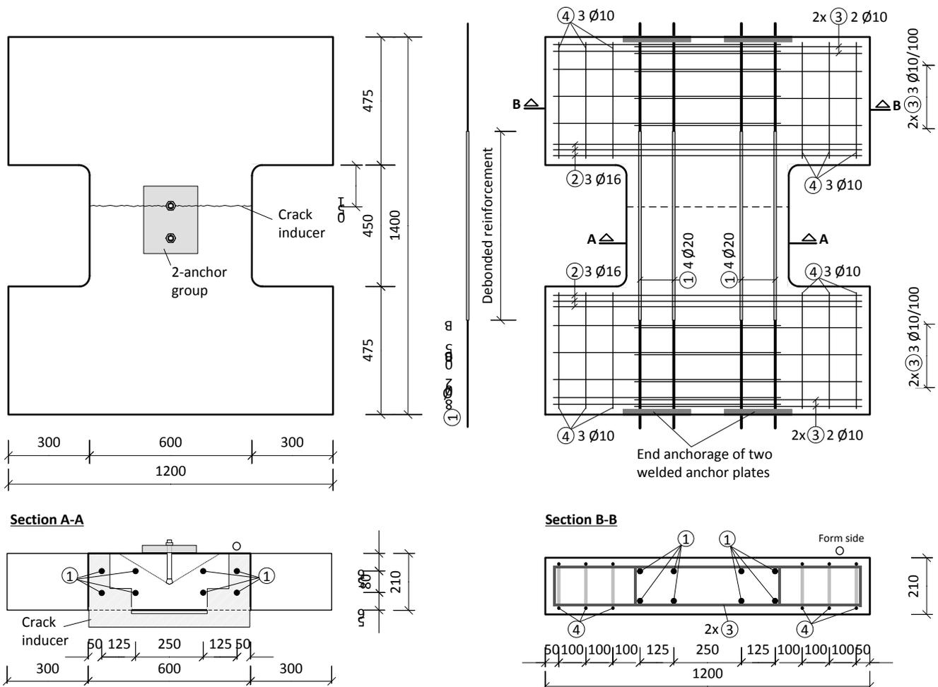
Fig. 3 – Drawing of concrete specimen (all units in mm)
