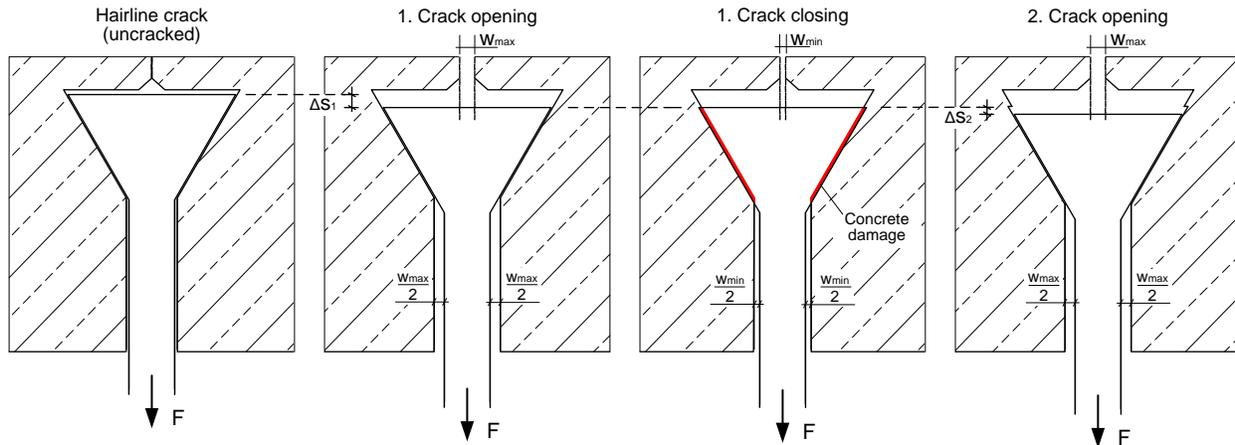
Fig. 9 – Load-displacement behavior of undercut anchors during crack cycling at constant load acc. to [7]
