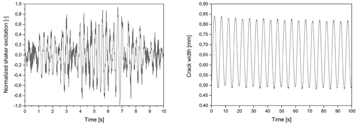
Fig. 5 – Normalized time history of shaker (left) and crack width during test 3.1, loading level  $\gamma_M N_{Rd}$  (right)
