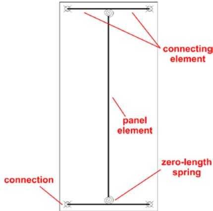
Fig. 10. Five beam model for panels with four connections.
