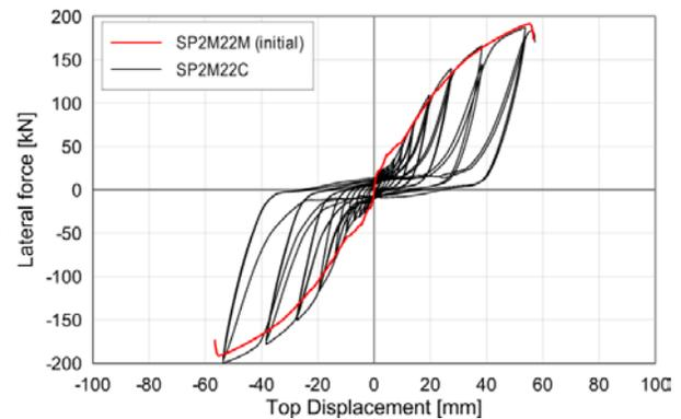
Fig. 7. Lateral force versus displacement relationship for connections with bolted plates (from [6]).
