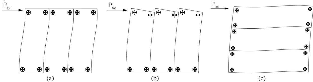
Fig. 1. Arrangement of panels: (a) Vertically with four fixed connections; (b) Vertically with two fixed and two sliding connections; (c) Horizontally with four fixed connections.
