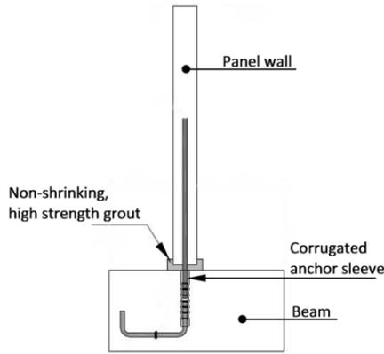
Fig. 2. Connection with protruding rebars.
