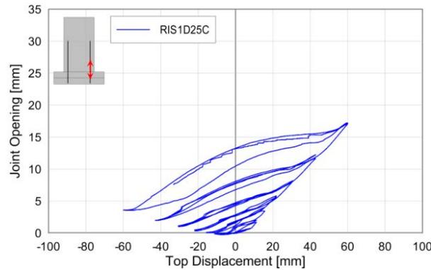
Fig. 9. Joint opening vs. top displacement for connections with protruding rebars (from [6]).
