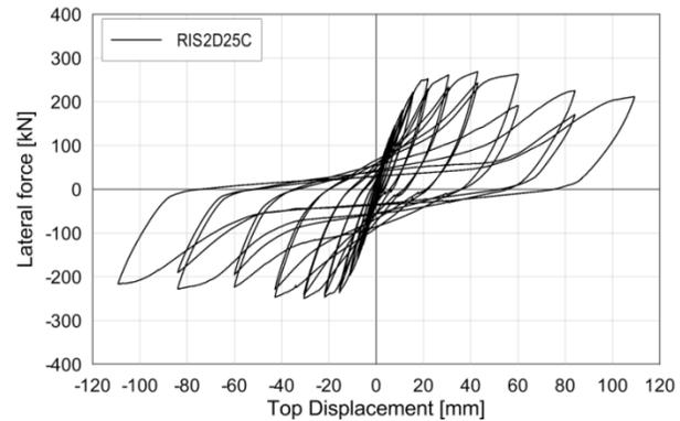
Fig. 3. Lateral force versus displacement relationship for connections with protruding rebars (from [6]).
