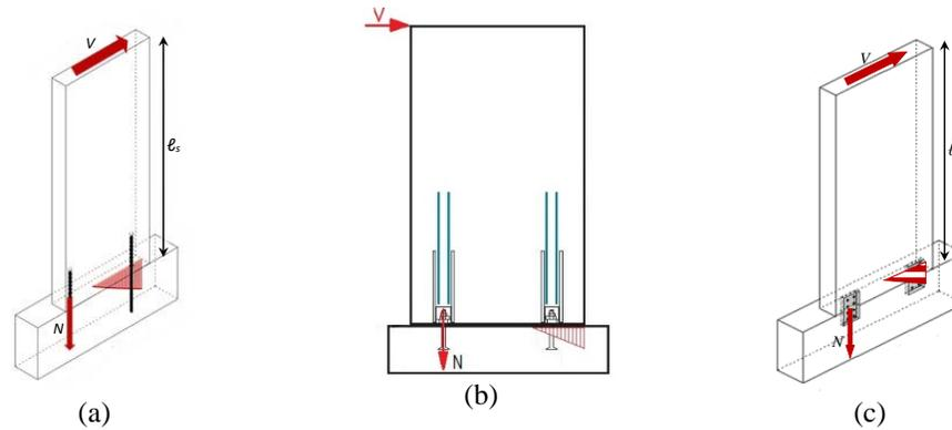
Fig. 8. Resisting mechanism for connections with: (a) Protruding rebars; (b) Bolted shoes; (c) Bolted plates.
