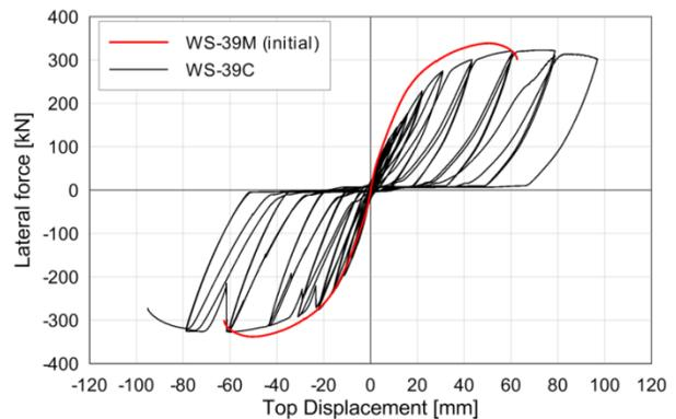
Fig. 5. Lateral force versus displacement relationship for connections with bolted shoes (from [6]).
