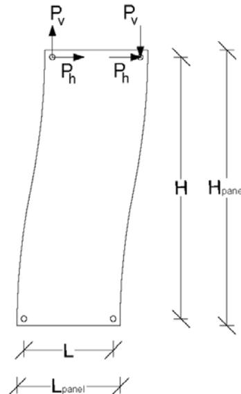
Fig. 12. Distribution of forces at a panel with four connections.
