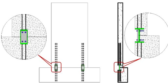
Fig. 6. Connections with bolted plates.
