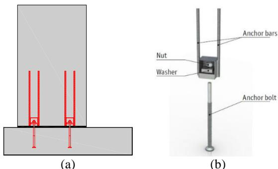
Fig. 4. Connections with bolted shoes: (a) Schematic view; (b) Wall shoe.
