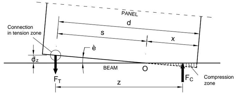
Fig. 11. Forces and rotation at the base of the panel.
