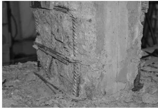
Fig. 13 – The damage of the specimen after the CFRP wrap was removed
