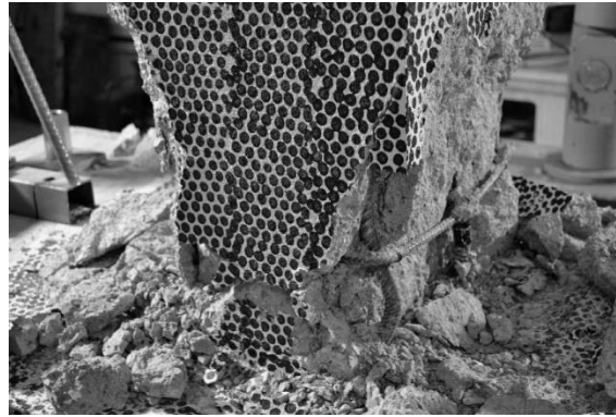
Fig. 5 – Significant damage of the concrete core and global buckling of longitudinal reinforcement after the second cycle at 6.40% drift amplitude
