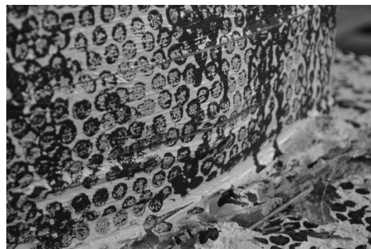
Fig. 11 – Modest rupture of CFRP wrap at 7.60% drift amplitude
