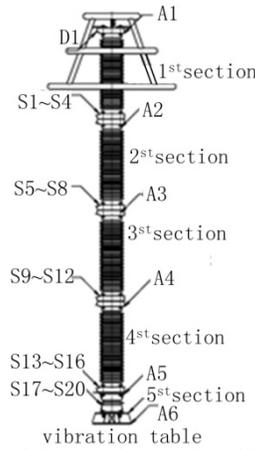
Fig. 5 – The schematic of the testing point distribution of equipment 1
