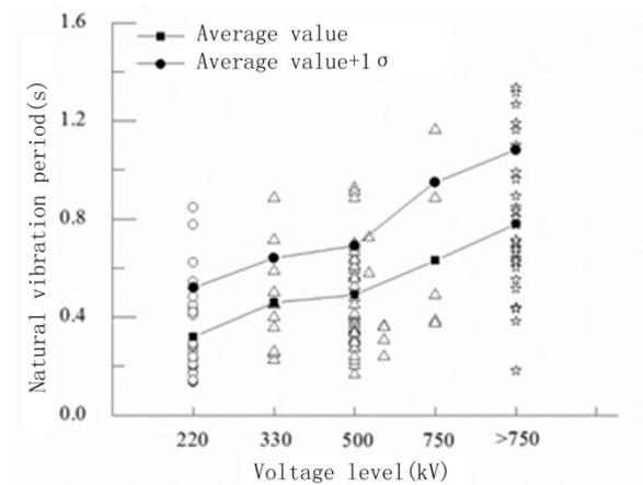
Fig. 2 – Relationship between natural vibration period of electrical equipments and the voltage level
