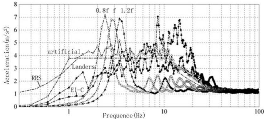
Fig. 9 –The response spectrums of output waves of the 750 kV insulator of Fuci
