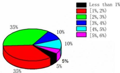
Fig. 3 – Damping ratio statistics of 500kV voltage level electrical equipments
