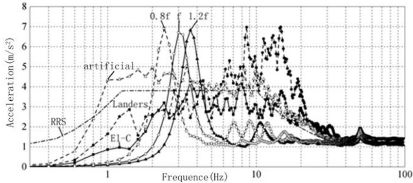
Fig. 8 –The response spectrums of output waves of the 500 kV arrester of Dongzhi
