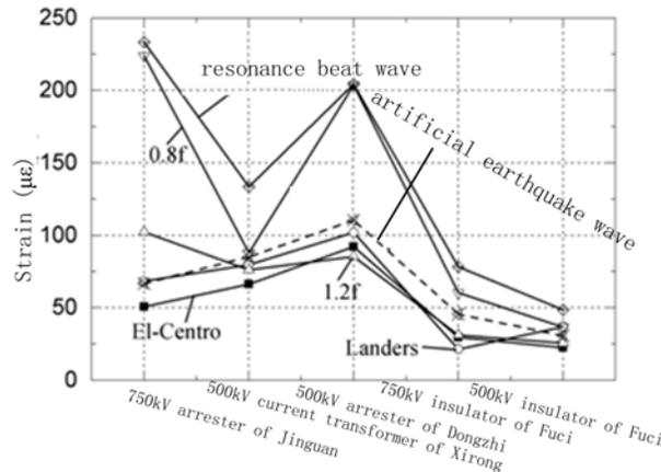
Fig. 7 – Peak strains (x direction) of the equipment bottoms under different seismic excitations
