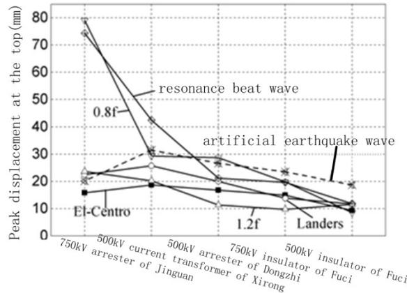
Fig. 6 – Peak displacement at the top of each equipment under different seismic excitations
