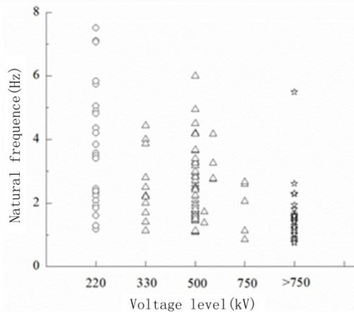
Fig. 1 – Relationship between natural frequency of electrical equipments and the voltage level
