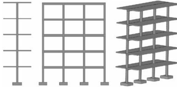
Fig. 1 – Schematic view of the five-story RC frame model: front (left), side (centre) and isometric view (right) without infills, adapted from Silva *et al.* [13].
