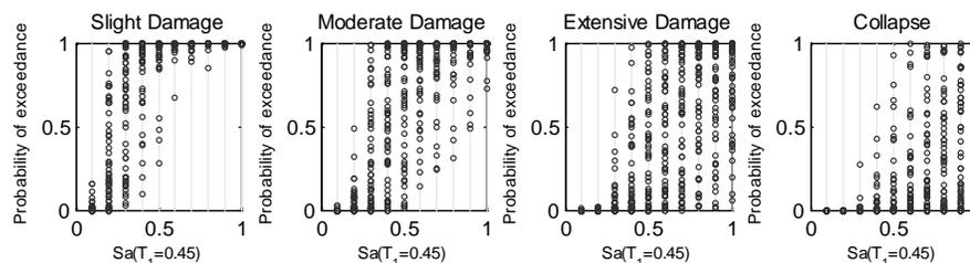
Fig. 3 – Record-specific probabilities of exceedance of *SD*, *MD*, *ED* and *Col*, as a function of *GD* criteria; for 5-story buildings.
