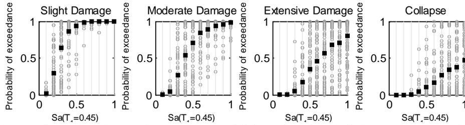
Fig. 5 – Record-specific probabilities of exceedance of *SD*, *MD*, *ED* and *Col*, as a function of *GD* criteria; and corresponding  $\tilde{P}ls_{i|Sa(T_1)=a}$  (illustrated by the black squares), for 5-story buildings.
