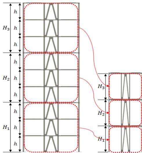
Fig. 4 – Scaling of the specimen
