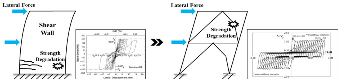
Fig. 6 – Lateral behavior of concrete shear walls and steel braced frames
