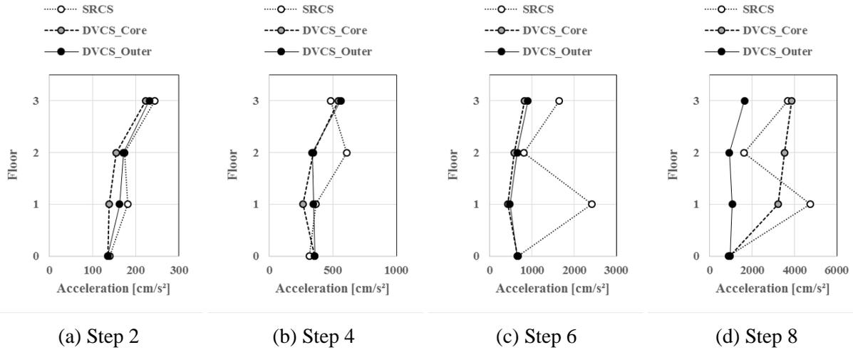
Fig. 9 – Maximum response acceleration of each floor
