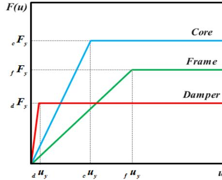
Fig. 2 – Restoring force characteristics of the DVCS
