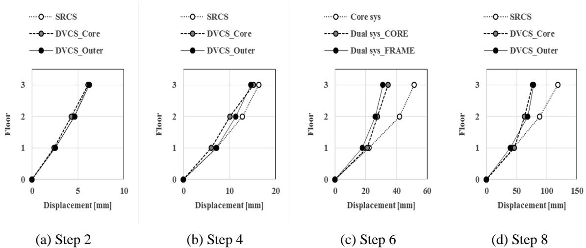
Fig. 11 – Maximum response displacement of each floor
