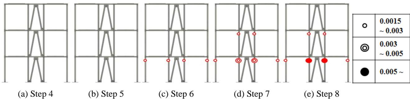
Fig. 12 – Damage distribution of the SRCS
