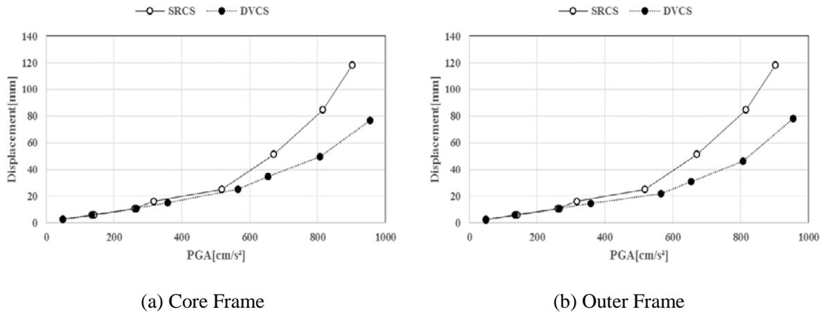
Fig. 10 – Maximum response displacement of both systems
