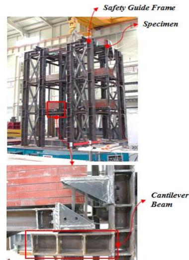
Fig. 5 – Setting up the specimen
