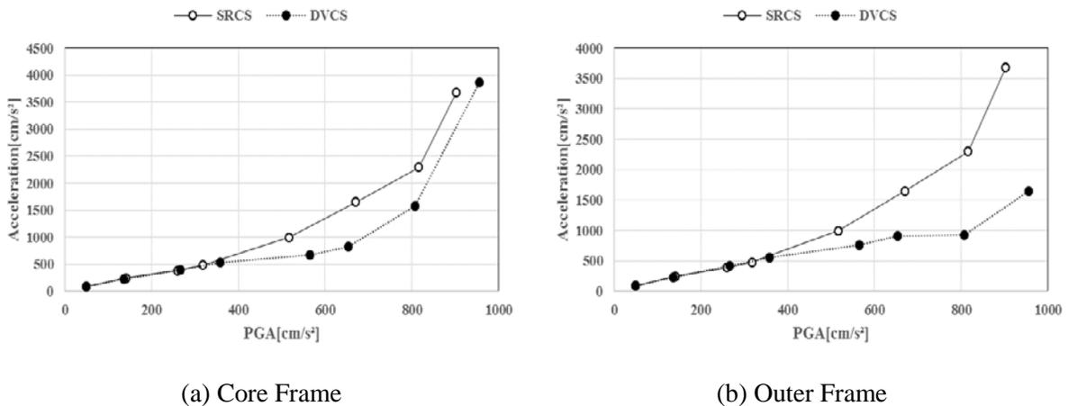
Fig. 8 – Maximum response acceleration of both systems
