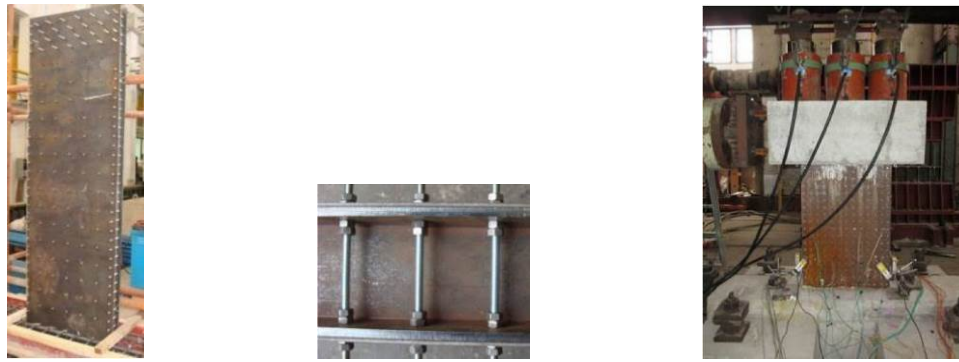
(b) Specimen construction (c) Bolt connection with eight nuts (d) Specimen installation
