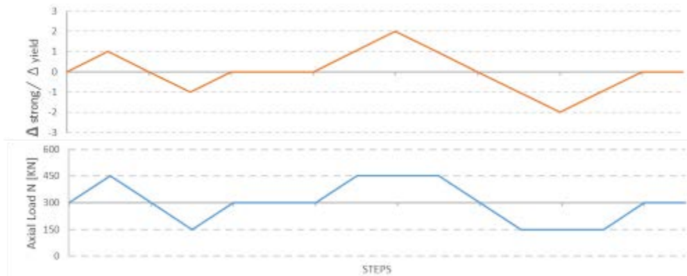
Fig. 2 – Applied axial load related to the strong direction displacement (*)
