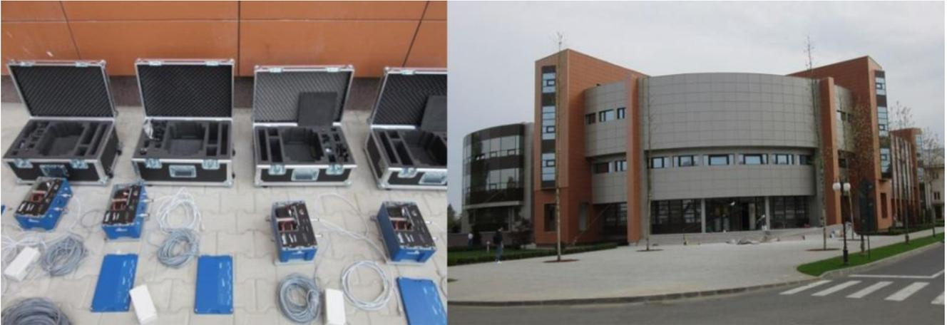
Fig. 8 – The acquisition system with four GMS Plus digital seismic stations used for temporary seismic instrumentation of the new building of Biology Faculty from Bucharest, B+G+2F (5 bays of 5.00 m and 5 openings of 5.00 m;  $H_{ground\ floor} = 3.80\ m$ ,  $H_{levels} = 4.10\ m$ )
