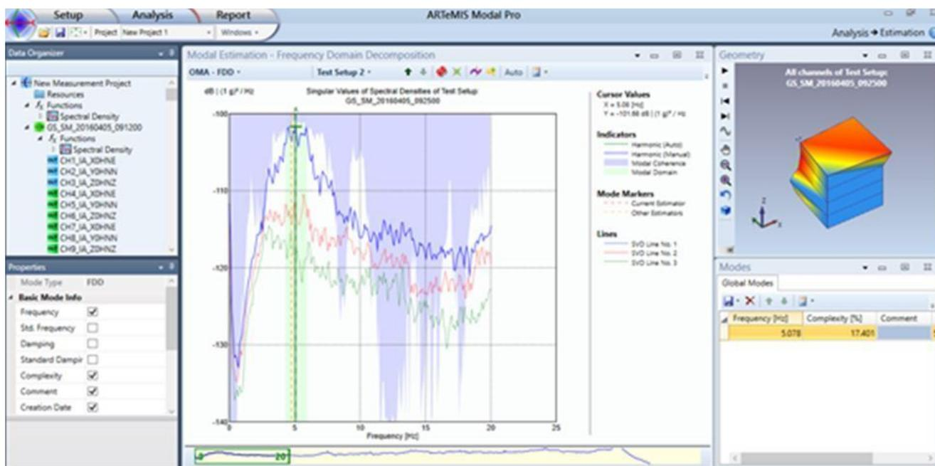
Fig. 11 – The results obtain following the Operational Modal Analysis, FDD technique
