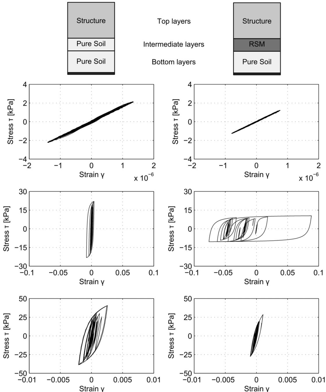
Fig. 4 – Comparison of the stress-strain response between the isolated and the non-isolated case when the system is subjected to Corralitos H2 seismic record. (Figure taken from [8])
