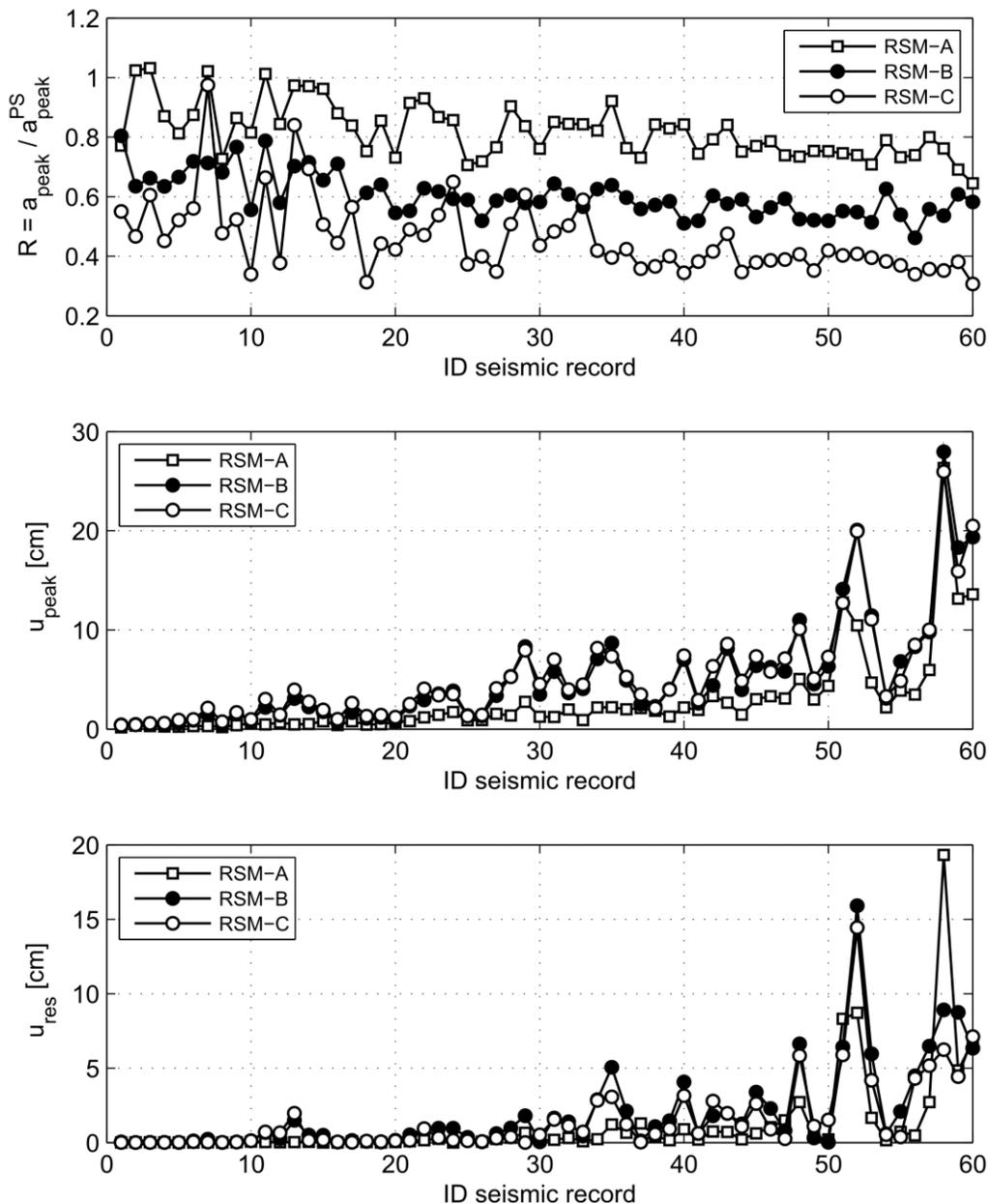
Fig. 6 – Acceleration reduction, peak displacement and residual displacement of the structure when varying the applied seismic record. (Figure taken from [8])
