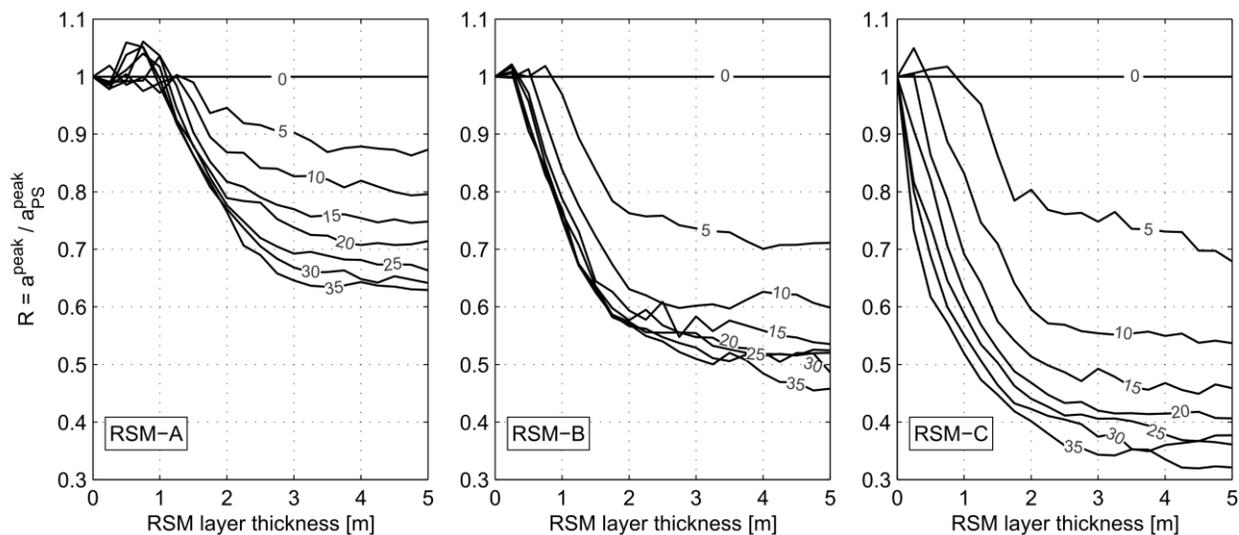
Fig. 7 – Peak acceleration measured at the bottom of the building normalized by the peak acceleration of the non-isolated case, when varying the thickness of the RSM layer. (Figure taken from [8])
