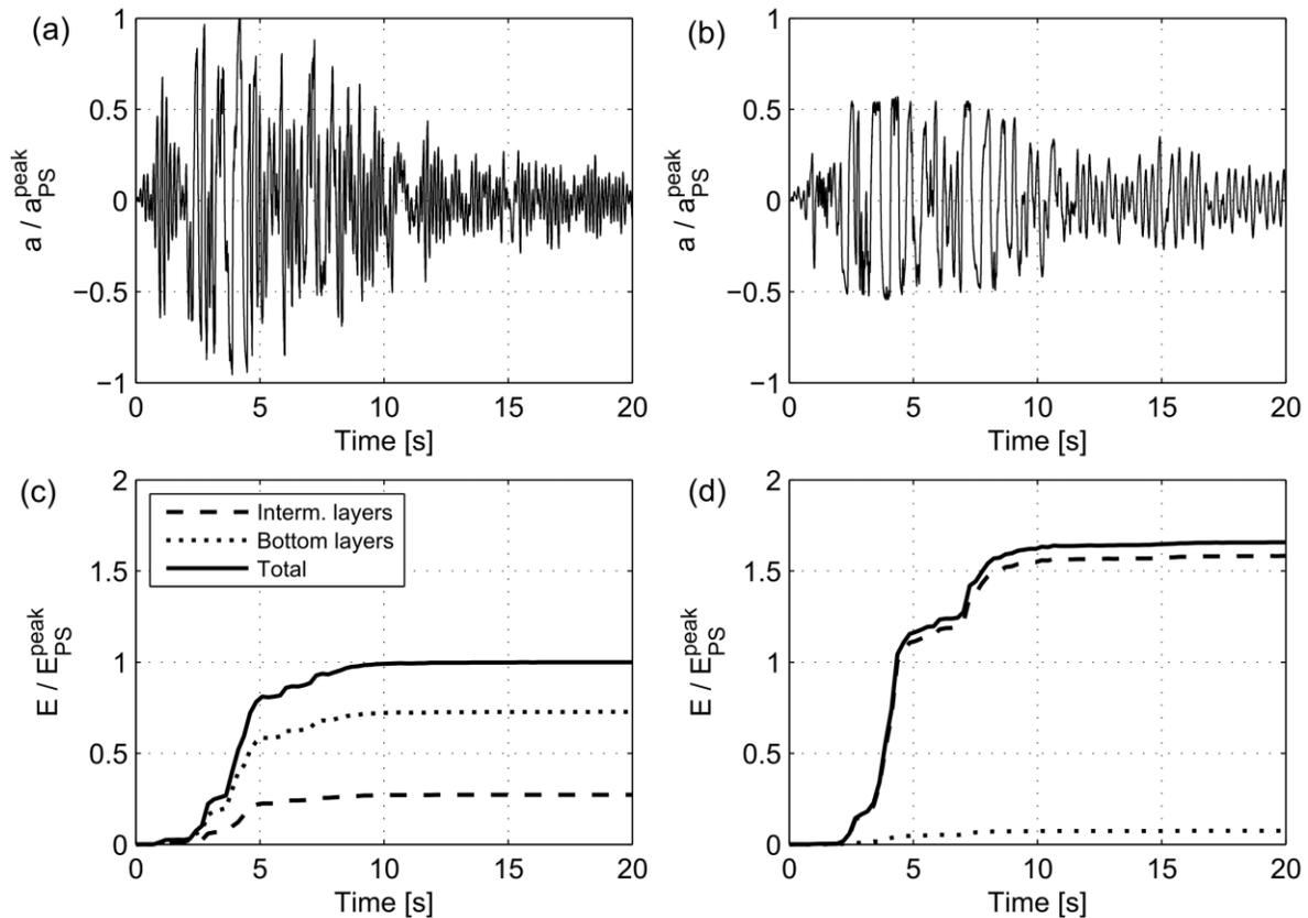
Fig. 5 – Comparison of the response of the system between the isolated and the non-isolated case, when it is subjected to the Corralitos H2 seismic record: (a) and (b) acceleration in the bottom of the building; (c) and (d) dissipated energy of the intermediate and bottom layers. (Figure taken from [\[8\]](#))
