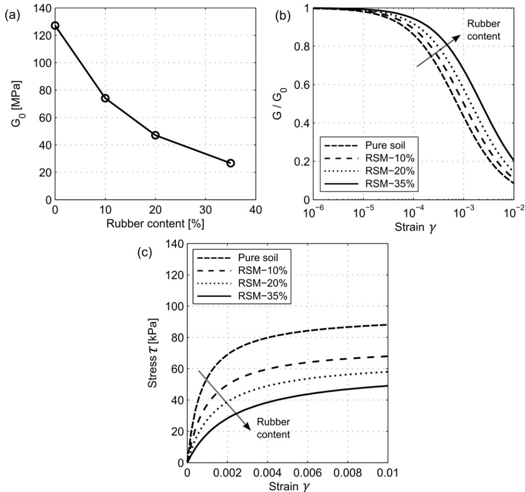
Fig. 1 – Effect of increasing rubber content in the shear properties of a typical soil (a) Initial shear modulus  $G_0$ ; (b) Shear stiffness degradation curve  $G/G_0$ ; (c) Stress-strain backbone curve. (Figure taken from [8])
