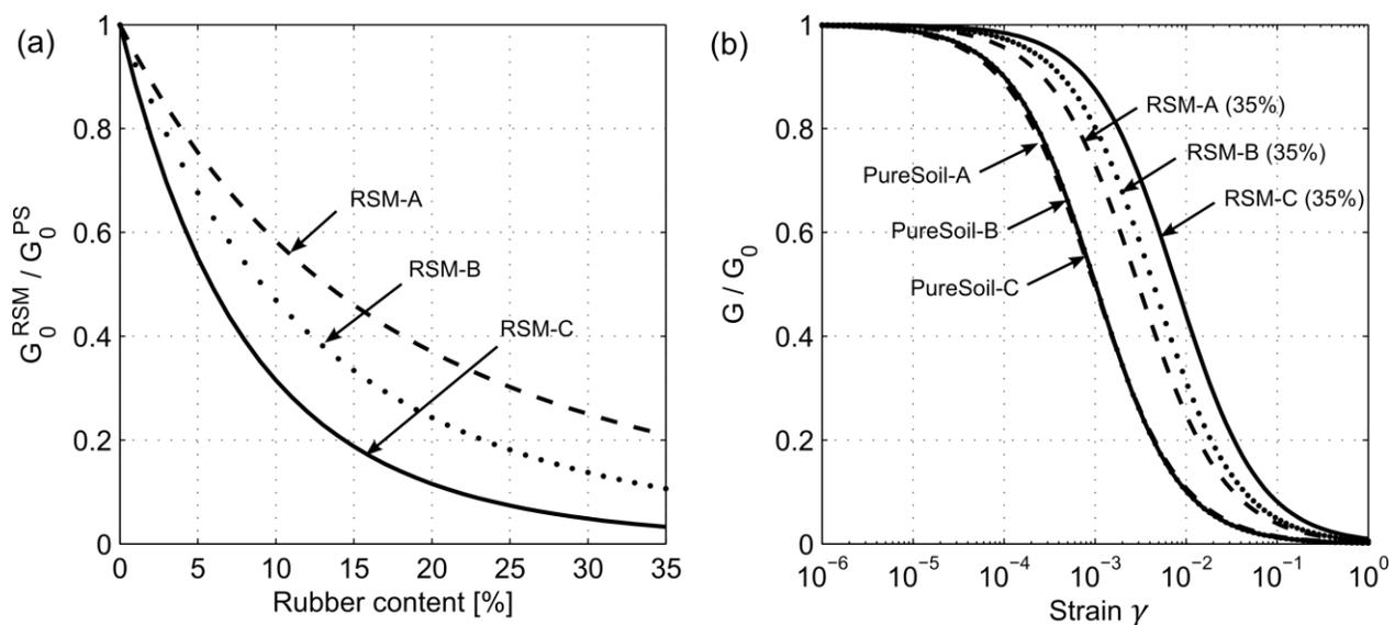
Fig. 2 – Pure soil and RSM curves used for analyses with  $\sigma_m=100$  kPa: (a) Ratio between small-strain shear moduli of the mix and the pure soil; (b) Stiffness degradation of pure soil and RSM with 35% rubber content. (Figure taken from [8])
