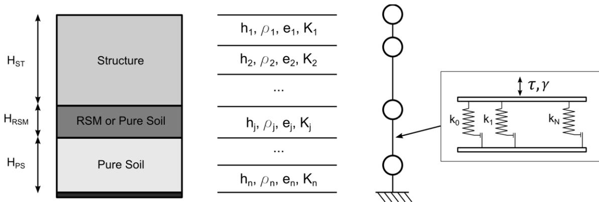
Fig. 3 – Idealization of the structure and soil profile as a multi degree of freedom system. (Figure taken from [8])
