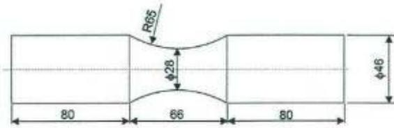
Figure 5. Shape and dimensions of test specimen (mm)
