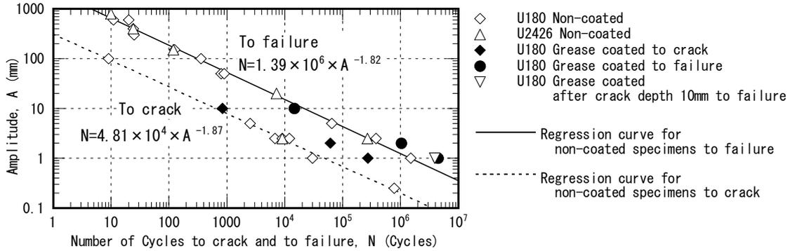
Figure 10. Relationship between amplitude and number of cycles
