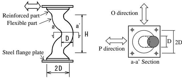
Figure 1. U-shaped lead damper
