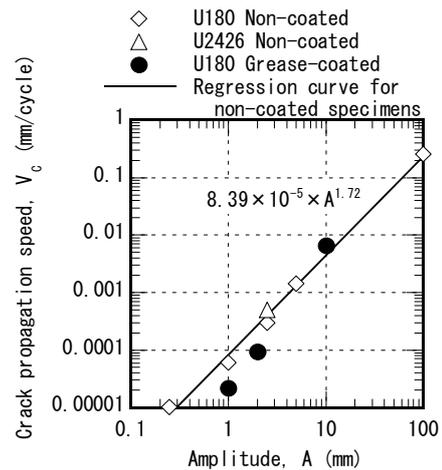
Figure 12. Relationship between crack propagation speed and amplitude
