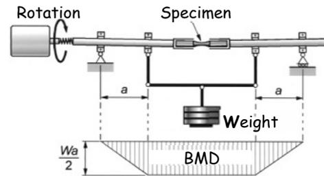
Figure 6. Rotating-bending fatigue test machine
