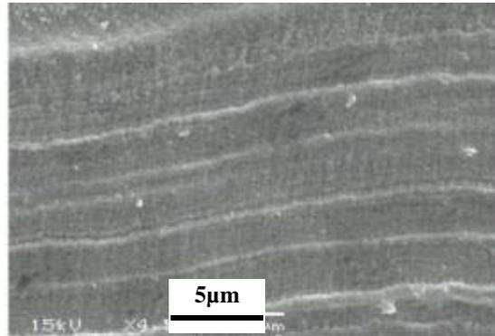
Figure 13. Fracture surface of a lead damper (4,500 magnifications)
