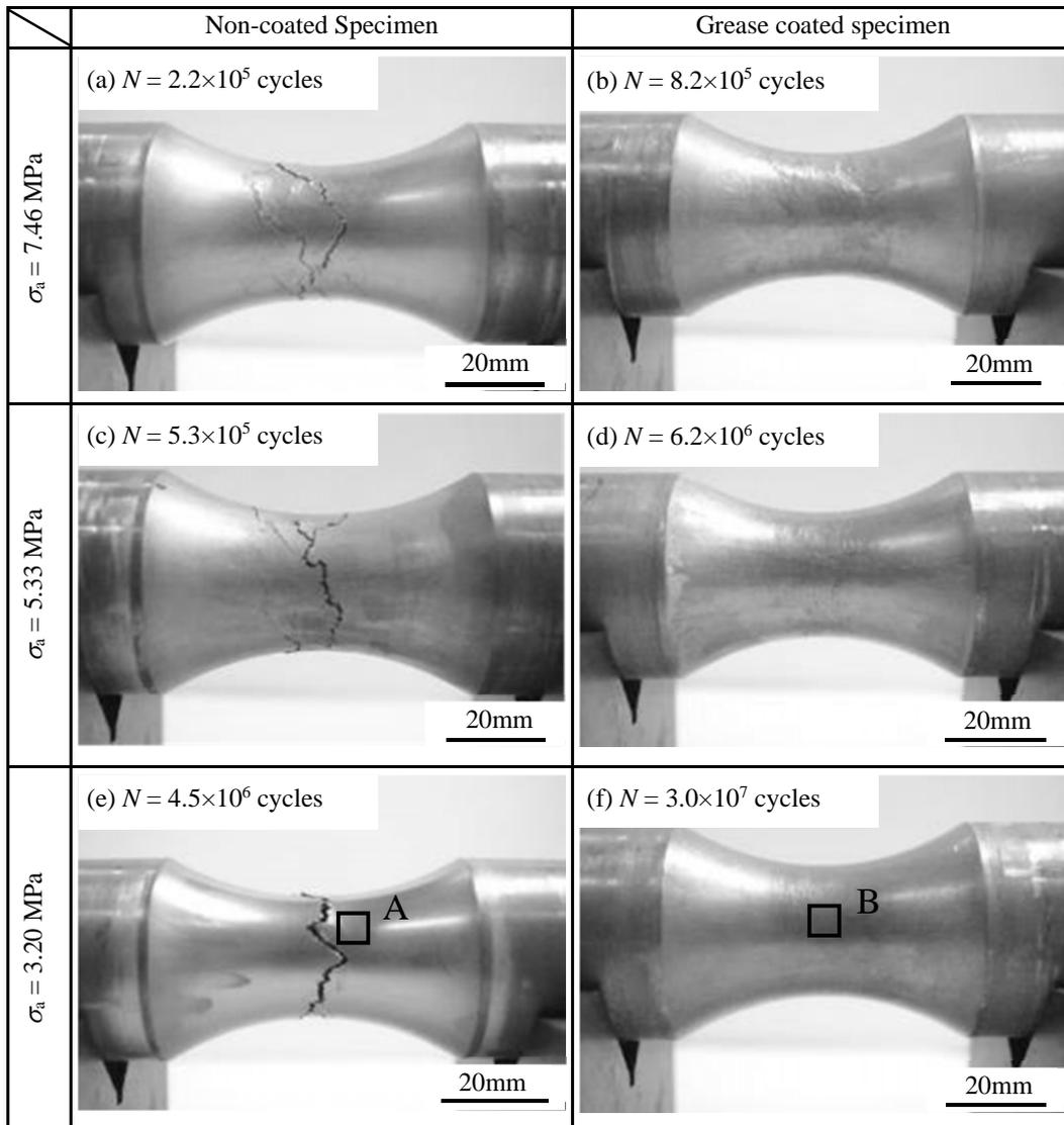
Figure 8. Photographs of the specimen surface after fatigue test
