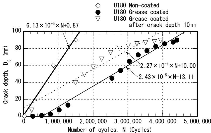
Figure 11. Relationship between crack depth and number of cycles
