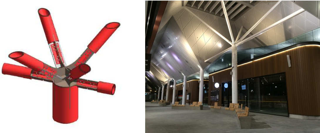
Fig. 7- Tree column details from REVIT and as built, left and right images respectively (REVIT 3D modelling detail and site photograph courtesy of Aurecon New Zealand).
