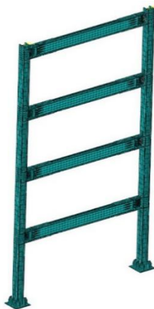
Fig. 5 The mesh generation of the ICSCSF model
