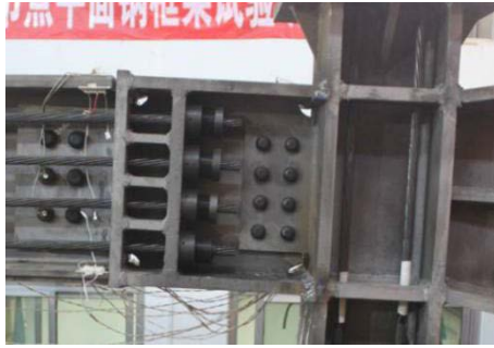
Fig.8 (a) The opening on western side is 14.04mm, the gap-opening is 2.23%
