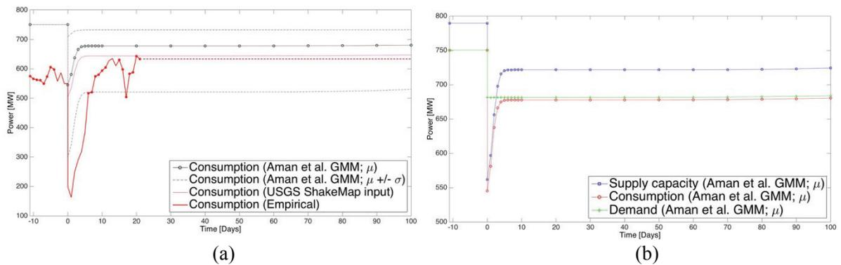
Fig. 4 – (a) Comparison of the empirical and simulated consumption curves (b) LoR using the ground motion model [30]
