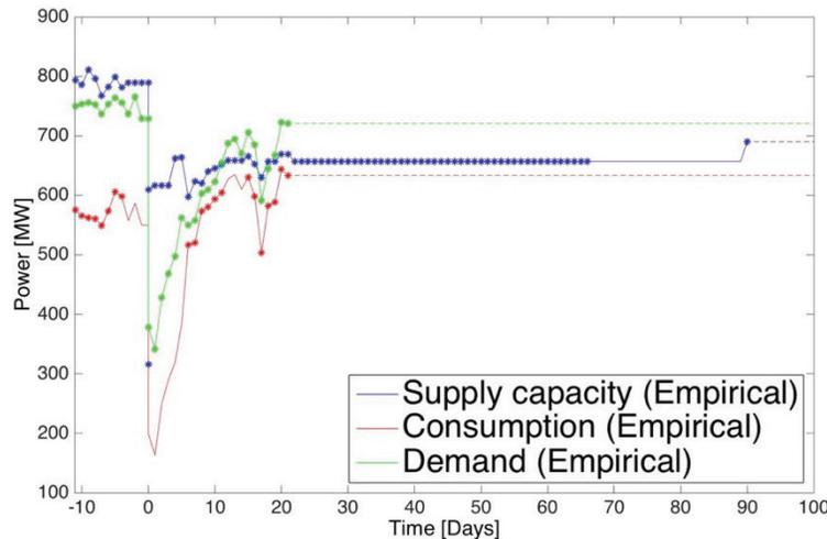
Fig. 2 - Observed average supply capacity, demand and consumption curves for the INPS
