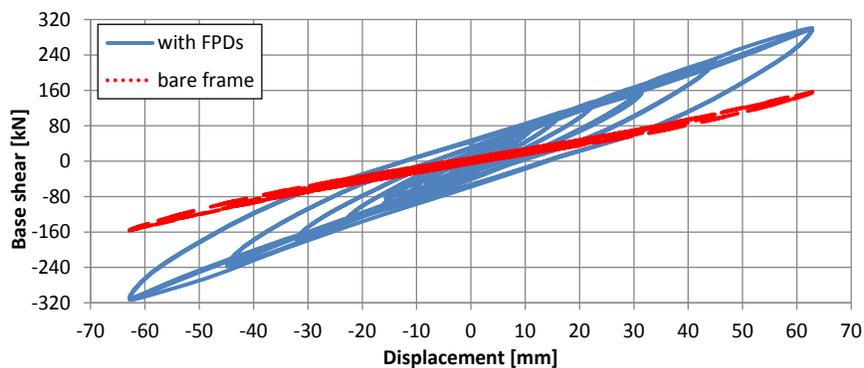
Fig. 8 – Full-scale cyclic tests: comparison of the base shear vs top displacement for the structural prototype with FPDs and the bare frame.
