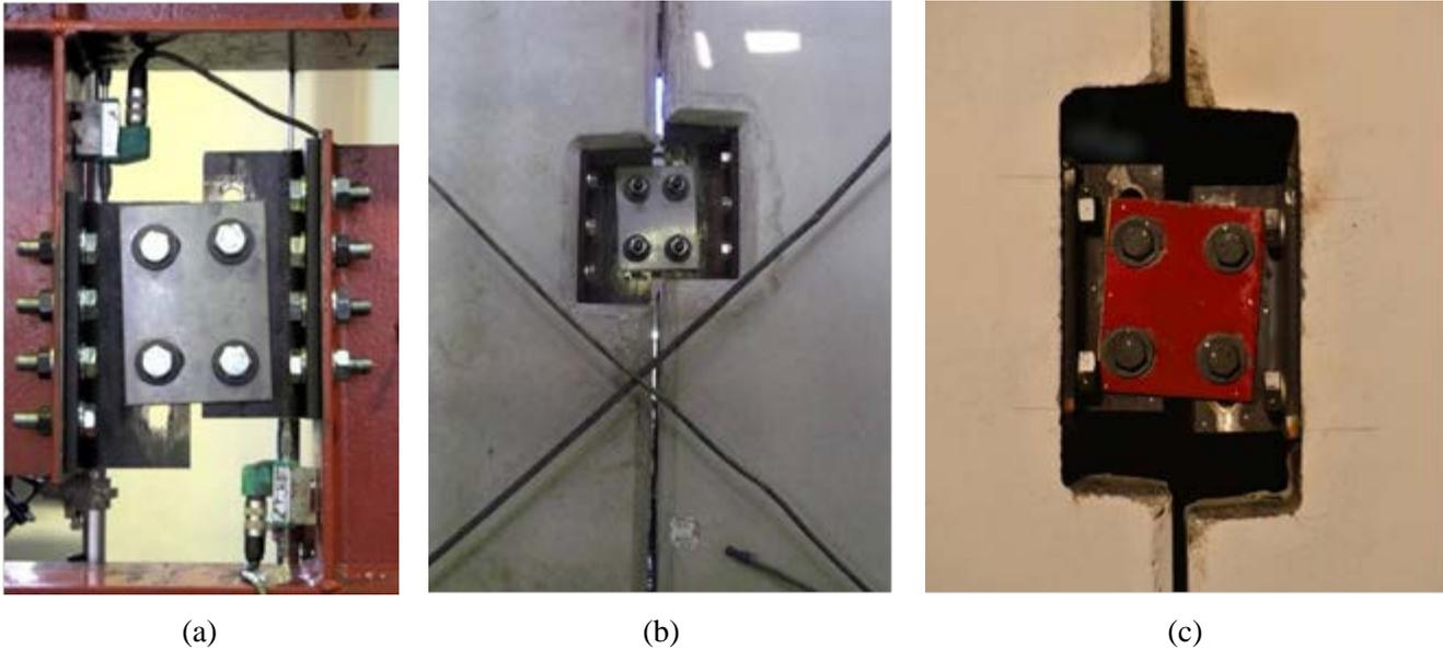
Fig. 17 – FBDs: configurations during (a) local tests, (b) sub-assembly tests, and (c) full-scale prototype tests.
