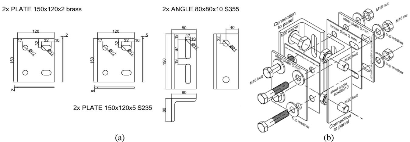
Fig. 3 - Friction Based Device (FBD) with angle supports: (a) geometrical dimensions of the components and (b) 3D view of the assemblage (courtesy of Marco Lamperti).
