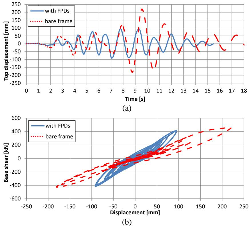
Fig. 9 - Full-scale pseudo-dynamic tests ( $PGA = 0.36g$ ): structural prototype with FPDs vs the bare frame in terms of (a) top displacement time history and (b) base shear vs top displacement.
