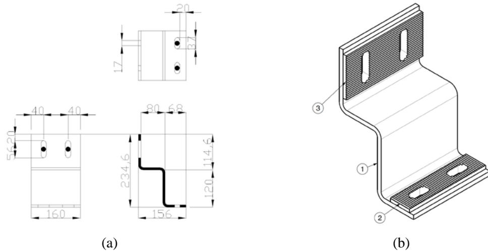
Fig. 1 – Folded Plate Device (FPD): (a) geometrical dimensions and (b) 3D view of the connector.
