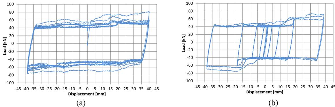
Fig. 13 - Local tests on FBDs: load vs displacement diagrams for (a) constant displacement amplitude protocol and (b) increasing displacement amplitude protocol.
