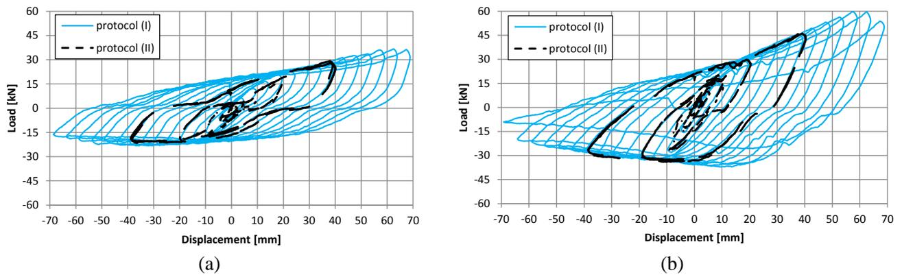
Fig. 6 – Local tests on FPDs: load vs displacement cycles for (a) unrestrained and (b) restrained out-of-plane displacement.
