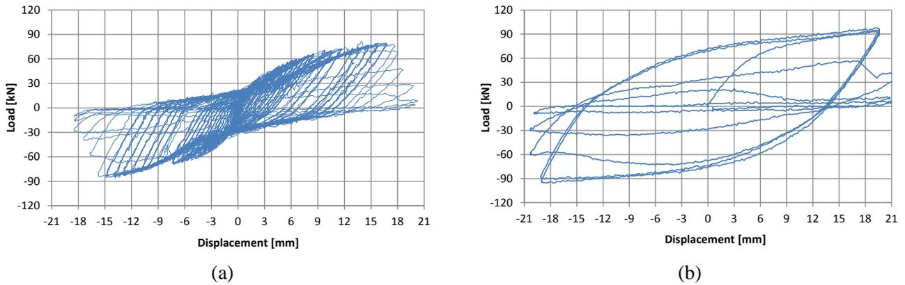
Fig. 10 - Local tests on MSDs: load vs displacement diagrams for (a) low-displacement and (b) large-displacement cyclic protocols.
