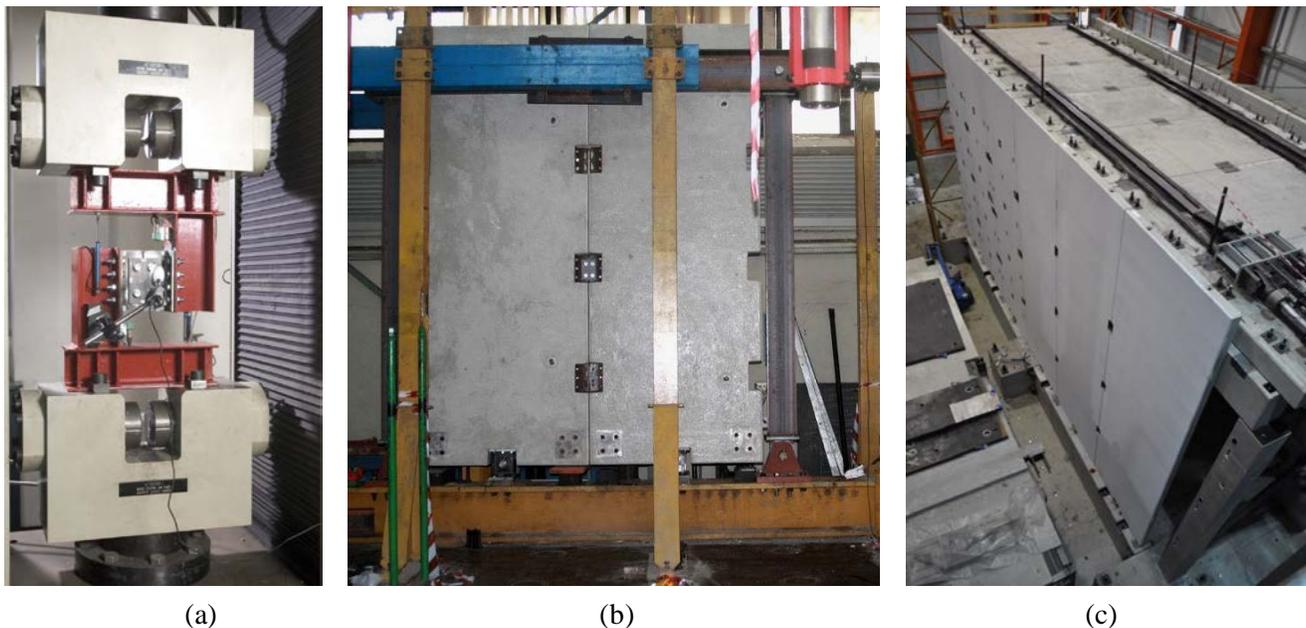
Fig. 5 - Test set-up: (a) local tests on single connectors; (b) sub-assembly tests; (c) full-scale prototype tests.
