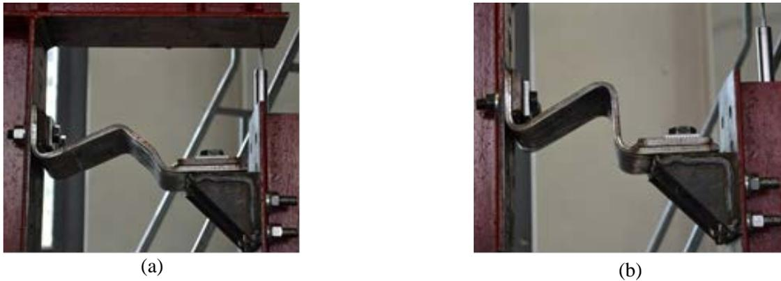
Fig. 7 - Local tests on FPDs: deformed configurations with large plastic deformation for (a) unrestrained and (b) restrained out-of-plane displacement.
