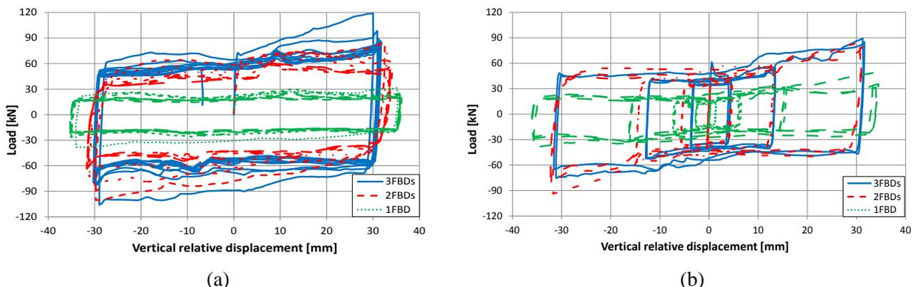
Fig. 14 - Sub-assembly tests on FBDs: load vs displacement diagrams for (a) constant displacement amplitude protocol and (b) increasing displacement amplitude protocol.
