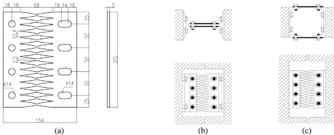
Fig. 2 – Multiple Slit Device (MSD): (a) multiple slit plate and assemblage on (b) T-shaped and (c) UPN profiles.
