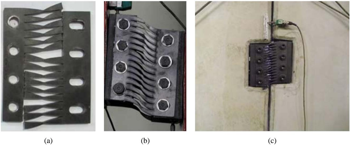
Fig. 11 – MSDs: (a) failure mode, and deformed configurations during (b) local test and (c) sub-assembly test.
