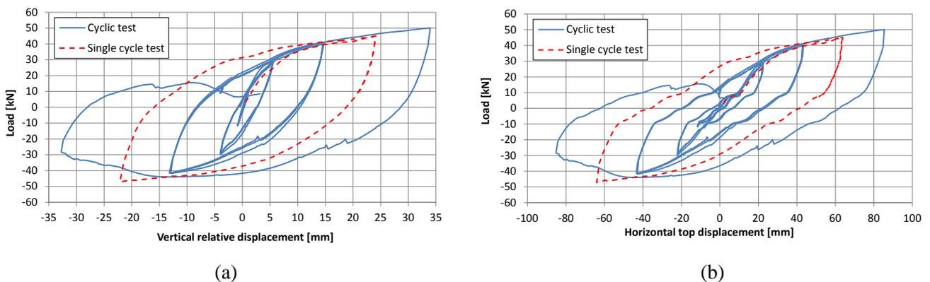
Fig. 12 - Sub-assembly tests on MSDs: (a) load vs vertical relative displacement, (b) load vs top displacement.
