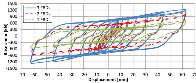
Fig. 15 - Full scale prototype cyclic tests on the structure with FBDs.
