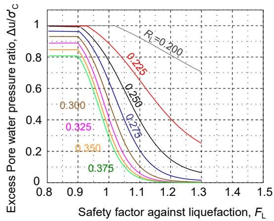
Fig. – 9 Relationship between  $F_L$  and excess pore-water pressure ratio used in this analysis
