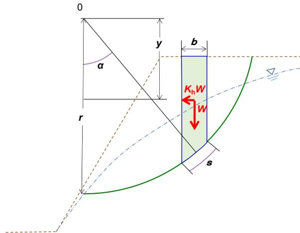
Fig. 2 – Stability analysis method introduced in the code
