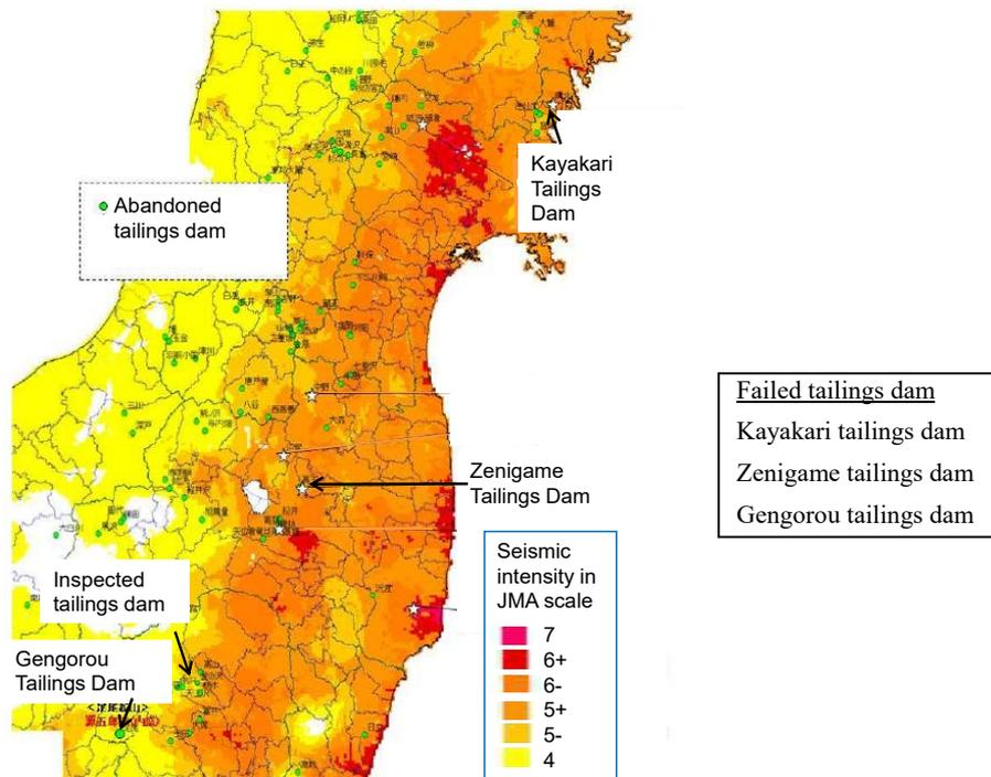
Fig. - 3 Locations of the three failed tailings dams and of tailings dams that did not fail (quoted from Technical Committee for Administration of Reservoir of Waste Soils and Tailings, 2012 [3])
