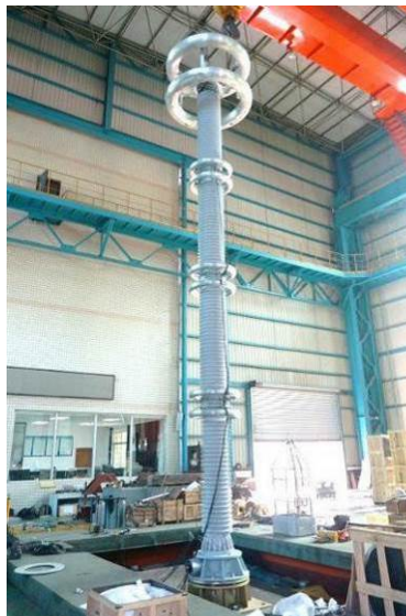
Fig. 12 Shaking table test of 1 000 kV capacitor voltage transformer
