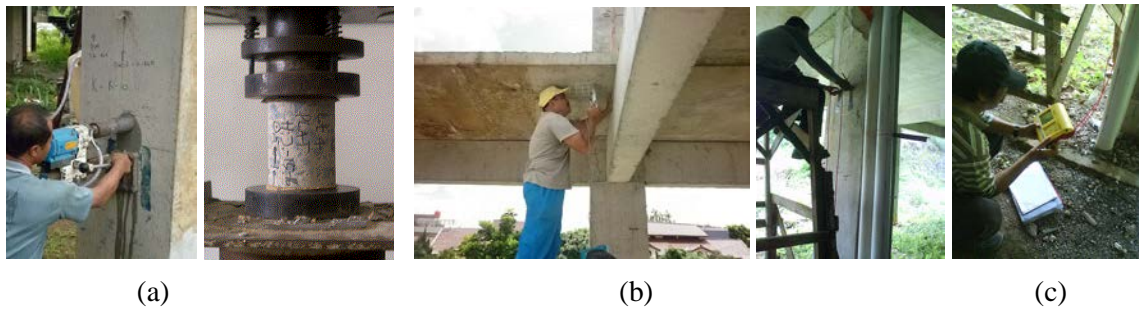
Figure 12 – Material testing: (a) core drill, (b) Schmidt hammer, (c) Ultrasonic Pulse Velocity
