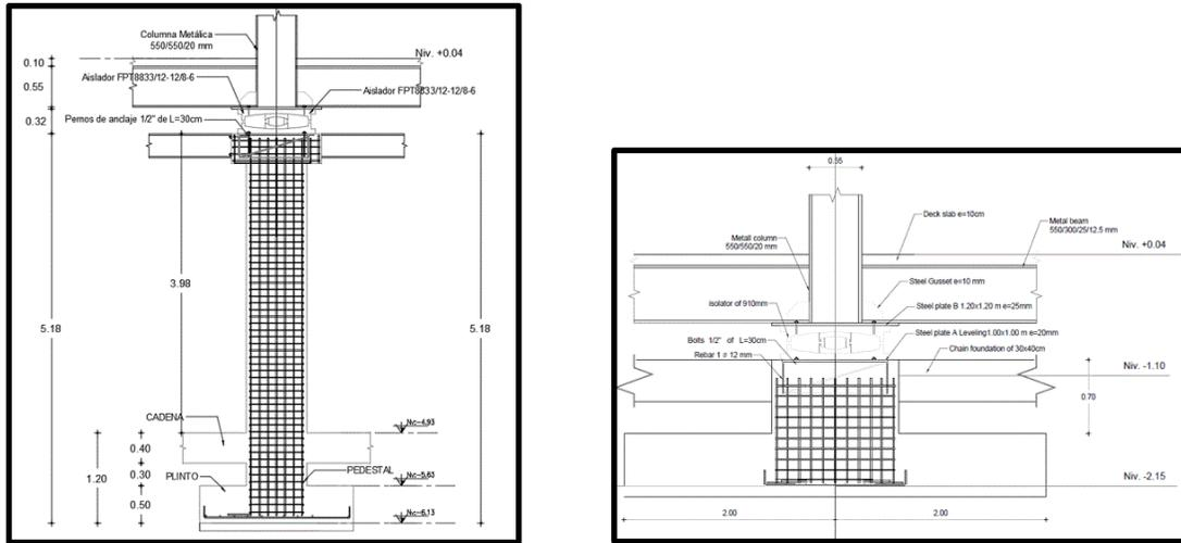
**Fig. 3** – FPT isolator on top of column and on top of pedestal. Source: Aguiar and Pazmiño (2016)
