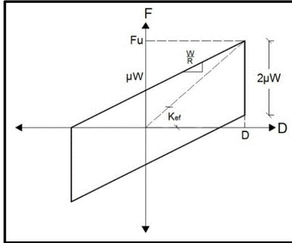
**Fig. 4 -** Bilinear constitutive model for the FPT isolator. Source: Mc Vitty y Constantinou (2015)
