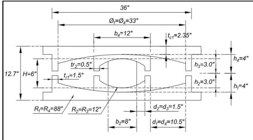
**Fig. 1** - Geometry of the triple friction pendulum isolator FTP8833 / 12-12 / 8-6
