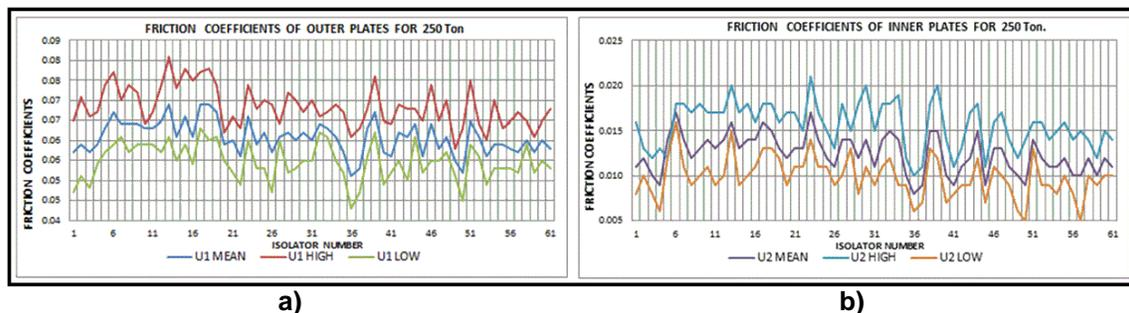
**Fig. 11** – Friction coefficients for 250 tonf: **a)** Exterior surfaces ( $\mu_1$ ): maximum, nominal and minimum values, **b)** Interior surfaces ( $\mu_2$ ): maximum, nominal and minimum values.
