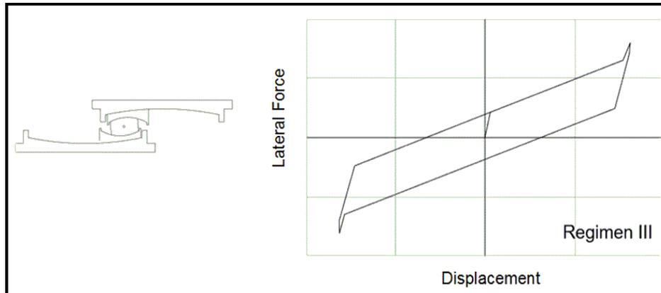
**Fig. 7** – Isolator performance in Regimen III. Source: Mc Vitty y Constantinou (2015)
