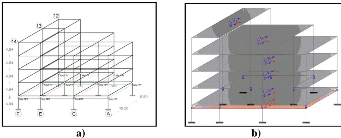
**Fig. 12 – Structural Block 3; a) Geometry and frame identification; b) Degrees of freedom used for the seismic analysis**
