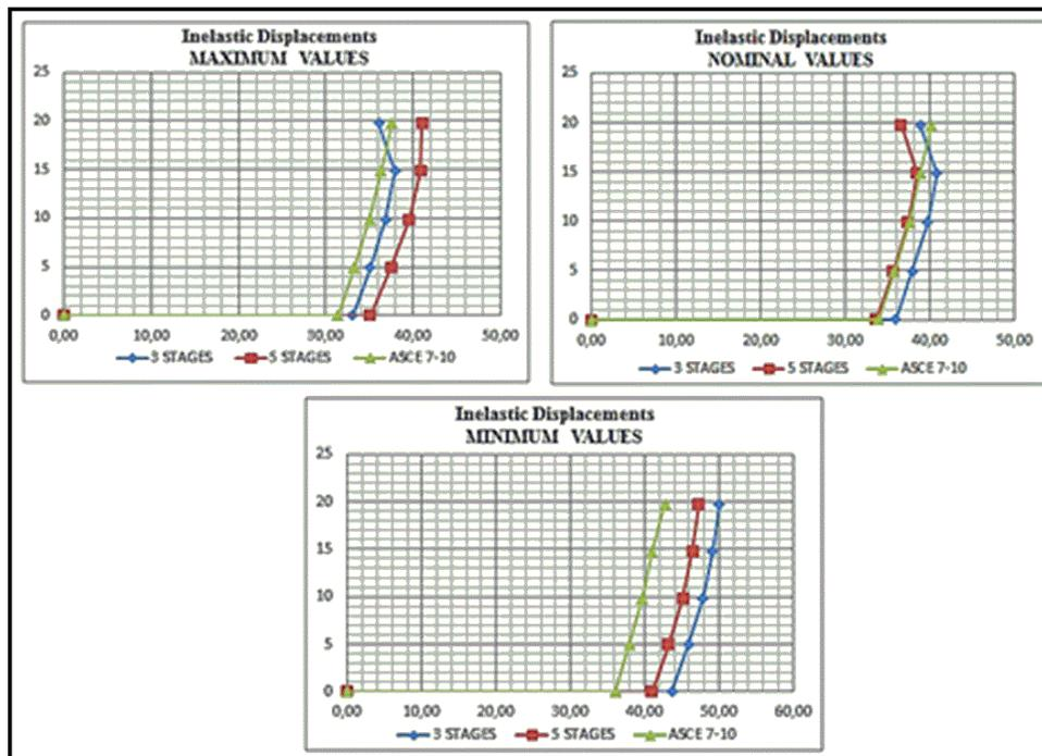
**Fig. 13** – Story displacements with maximum, nominal and minimum friction coefficient values
