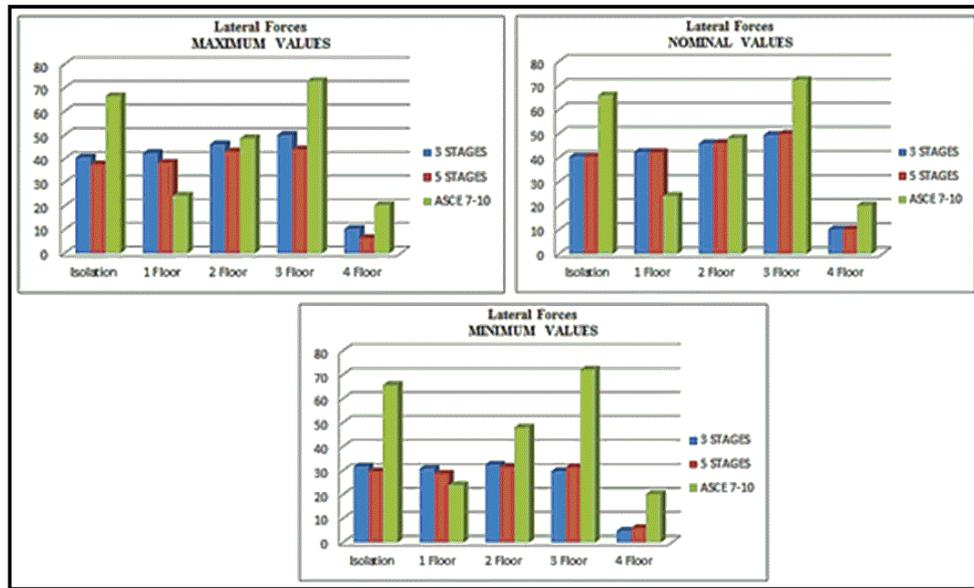
Fig. 14 – Story lateral forces with maximum, nominal and minimum friction coefficient values
