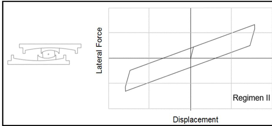
**Fig. 6** – Isolator performance in Regimen II. Source: Mc Vitty y Constantinou (2015)
