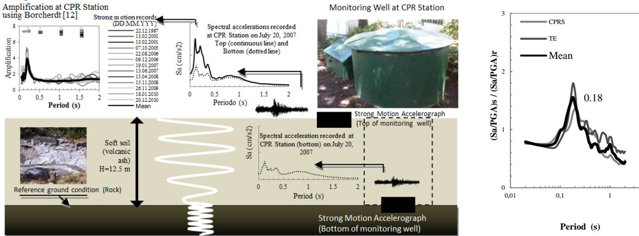
Fig. 4 – Left: Amplification due to local site condition at a Monitoring Well at “Casa Presidencial” Strong Motion Station (CPR) located just outside Santa Tecla) using Borchardt [12]. Right: Results using normalized response spectrum ratios at sites with similar surface geology: CPR Station outside Santa Tecla and Santa Tecla Strong Motion Station (TE) located in the Santa Tecla City Center.
