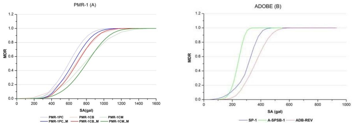
Fig. 9 – Vulnerability curves for: (A) single storey, reinforced masonry wall structure (PMR); PC, CB and CM stand for Pre-code, low code and medium code, respectively; M indicates the vulnerability curves developed in the present work; and (B) Adobe, SP-1 is related to precarious structures and A-SPSB-1 is the curve assigned to single storey adobe structures by a previous project whilst ADB-REV is the adobe vulnerability curve developed in the present work.
