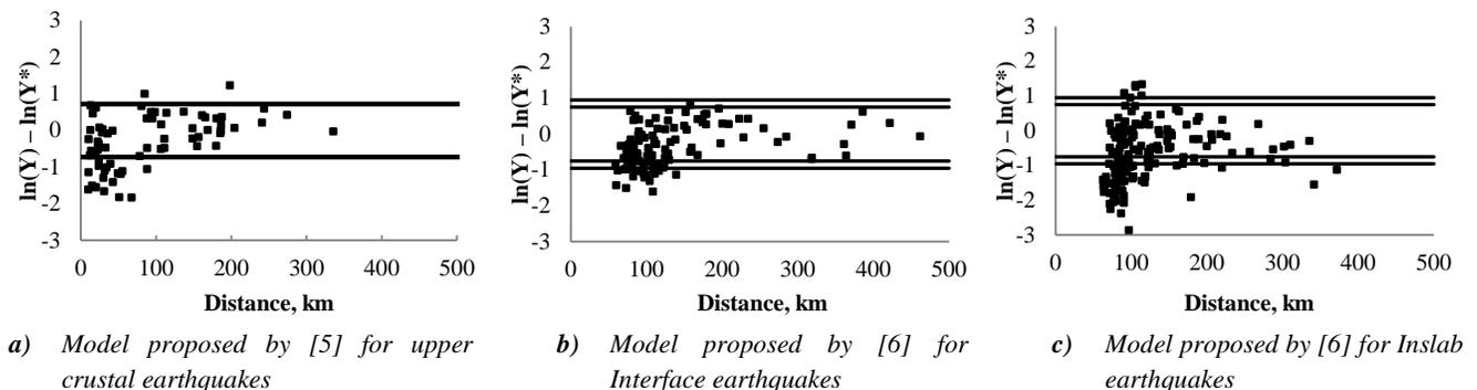
Fig. 2 - Distribution of R against distance for PGA for the models that show the best fit. The dots represent R and the solid lines represent the standard deviation established by each model
