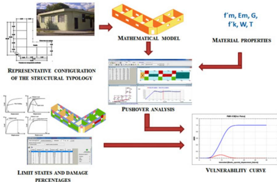
Fig. 7 – Schematic procedure for the development of vulnerability curves.
