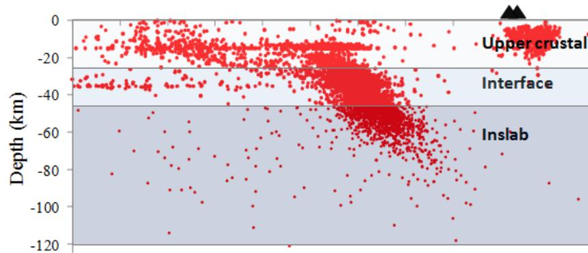
Fig. 1 – In Depth profile of El Salvador’s earthquake hypocenters from 1992 to 2012 and seismogenic zonation adopted for the seismic hazard assessment, with three tectonic regimes: upper crustal (<25 km), subduction interface (25<h<45) and subduction inslab (>45 km).
