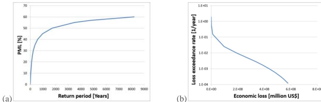
Fig. 10 – (a) Probable Maximum Loss (PML), (b) Loss Exceedance Curve
