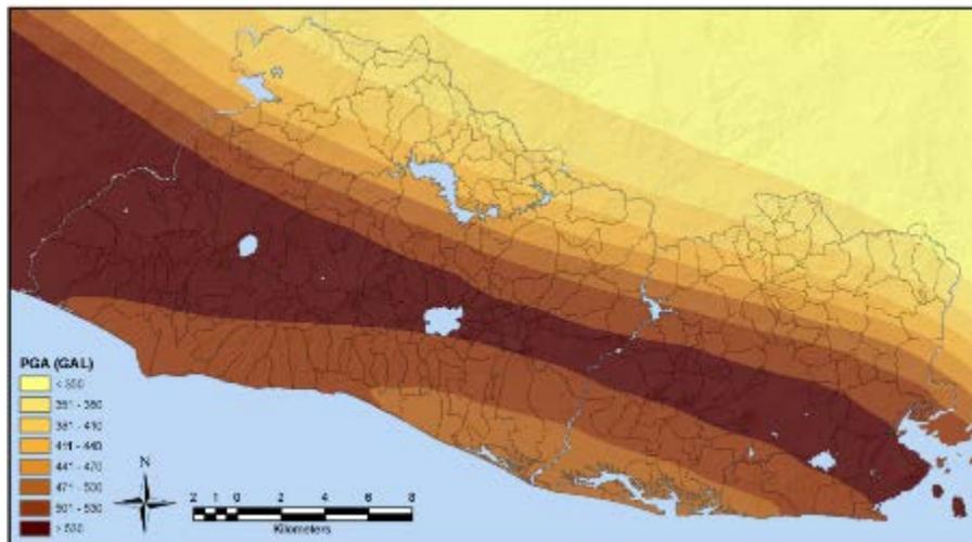
Fig. 3 – Seismic Hazard map of El Salvador, in terms of PGA (gal) for a return period of 500 years obtained in this study.
